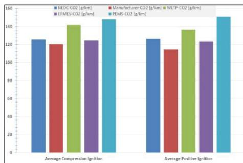
Fig. 1 Average CO<sub>2</sub> emission in g/km for cars with compression ignition and positive ignition engines.
