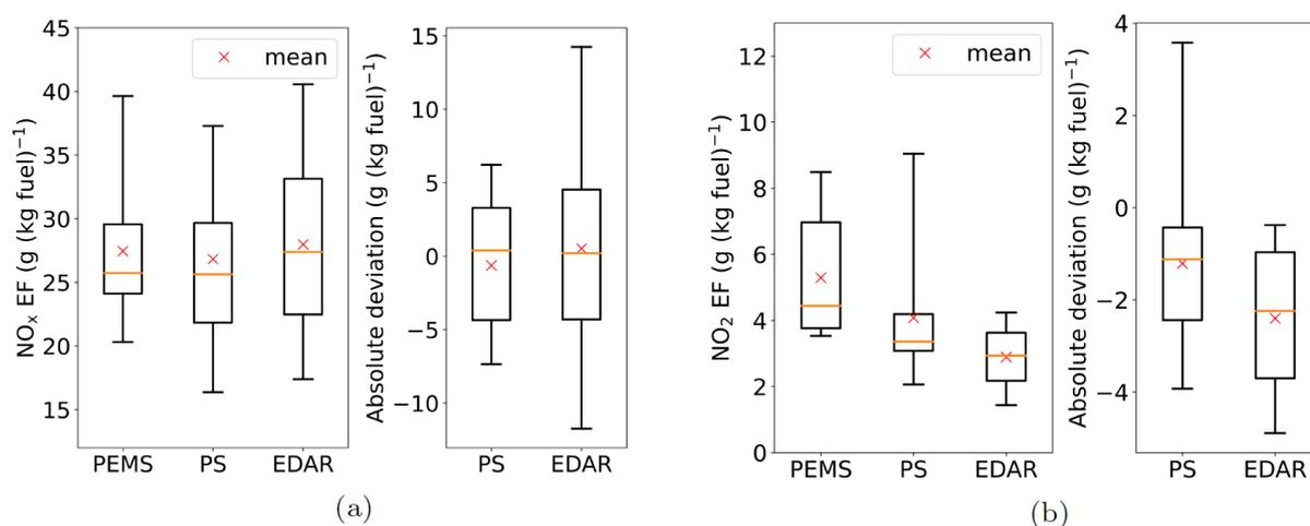
Figure 1. (a) Comparison of NO<sub>x</sub>-fuel-based emission factors (EFs) measured with PEMS, RES Type 2 (point sampling [PS]) and RES Type 1 (emissions detection and reporting [EDAR]). Left: Boxplots of the EFs. Right: Deviation of PS and EDAR measurements compared to PEMS. (b) Comparison of fuel-based NO<sub>2</sub> EFs measured with PEMS, PS, and EDAR. Left: Boxplots of the EFs. Right: Deviation of PS and EDAR measurements compared to PEMS.
