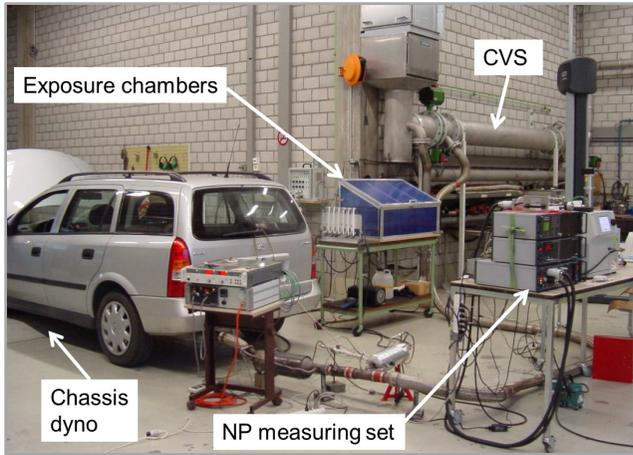
Fig. 1 Exposure Tests on a Diesel Passenger Car
