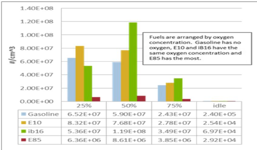
Fig. 2 Total Particulate Concentrations (#/cm<sup>3</sup>): 2.2-Liter DISI Engine
