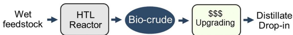
*Figure 42 Bio-intermediate production schematic via fast pyrolysis and hydrothermal liquefaction.*
