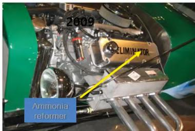
Oct '09 Ammonia Fueled V-8 with Hydrogen Injection: Reformed from NH<sub>3</sub>
