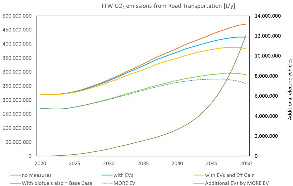
Figure 41: TTW CO<sub>2</sub> emissions in road transport by different measures for Brazil in the MORE EV scenario.
