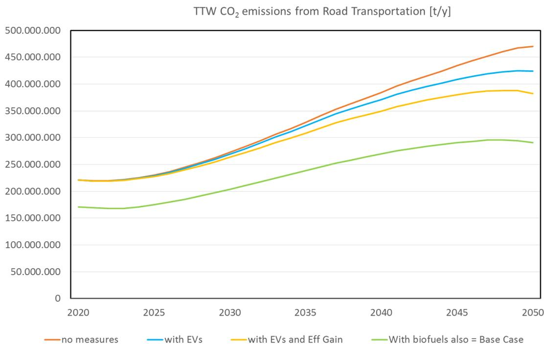
Figure 28: TTW CO<sub>2</sub> emissions in road transport by different measures for Brazil in the Current Policies scenario.
