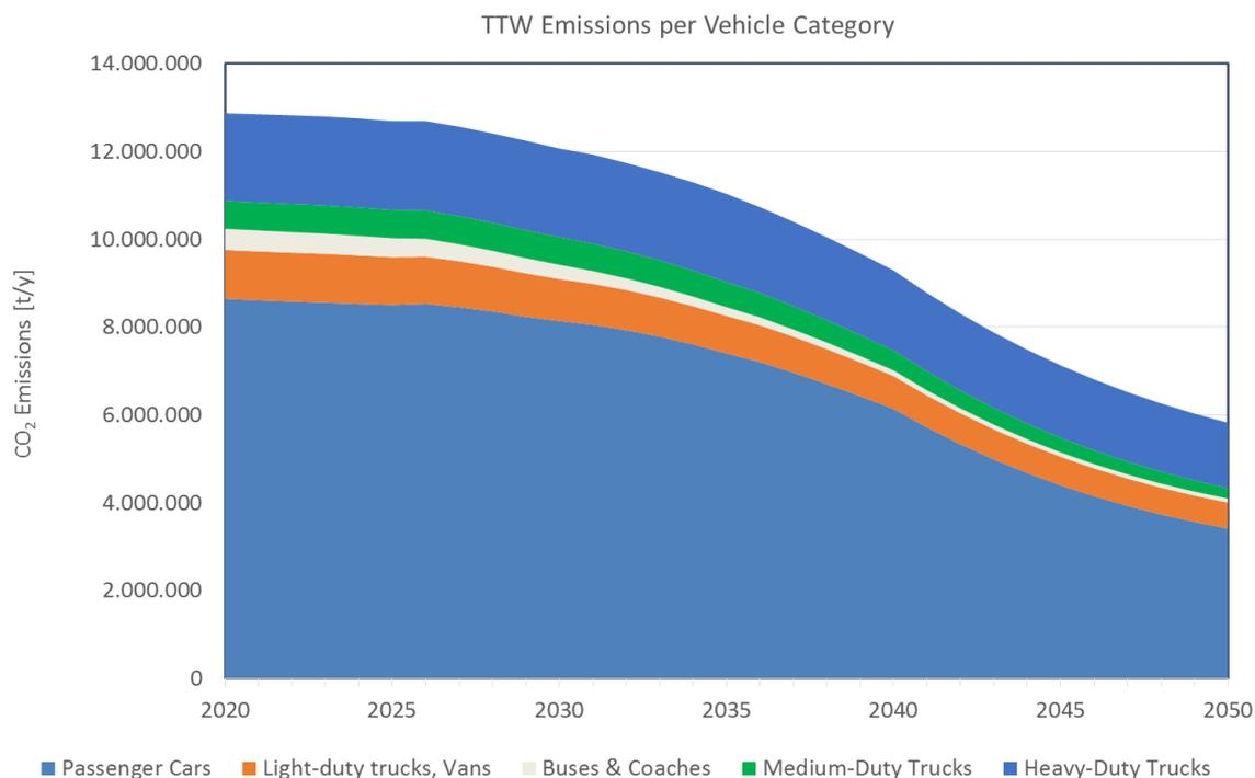
Figure 17: TTW CO<sub>2</sub> emissions in road transport by vehicle category for Sweden in the Current Policies scenario.
