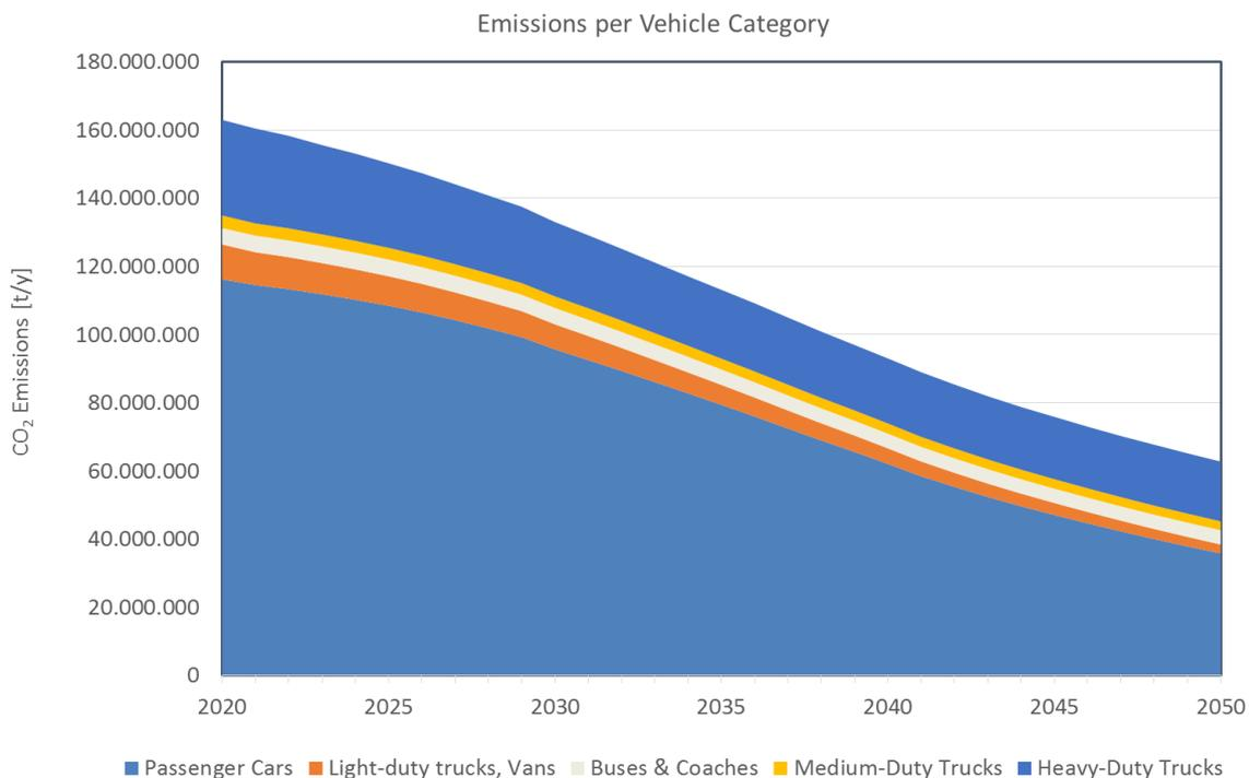
Figure 22: CO<sub>2</sub> Emissions in road transport by vehicle category for Germany in the Current Policies scenario.
