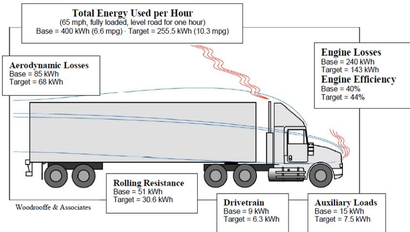
Figure 11: Energy audit for a conventional (MY 2000) Class 8 combination tractor (Bradley, 2000).
