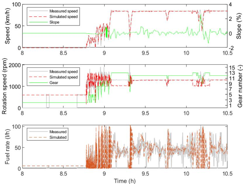
**Figure 31: Measured and simulated values for the simulation model validation: vehicle speed, engine speed and fuel rate.**
