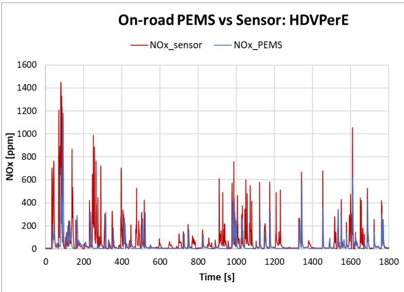
**Figure 84: Comparison of PROCARE Drive and PEMS devices for NO<sub>x</sub> concentrations. On-road test following the HDVPerE cycle.**
