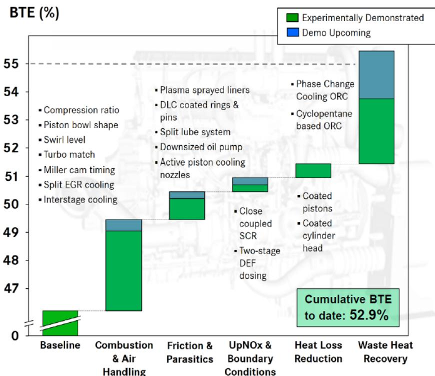
**Figure 15: Steps towards 55 % engine efficiency (Villeneuve and Girbach, 2020).**
