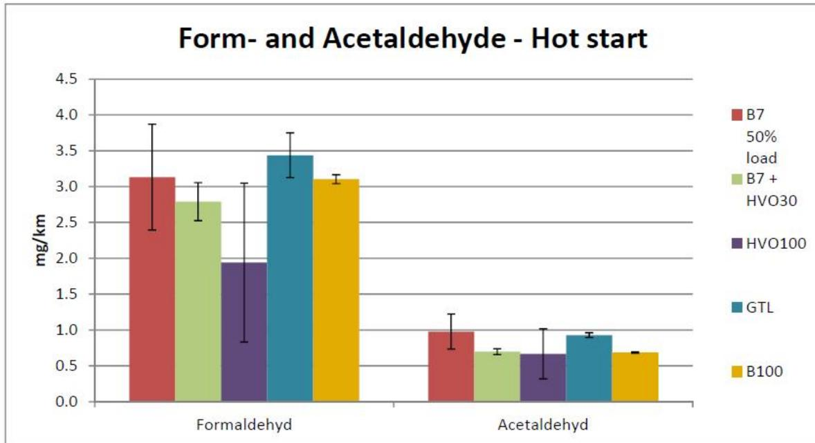
Figure 8.5 Formaldehyde and acetaldehyde emissions, diesel fuels, averaged results from hot start tests.
