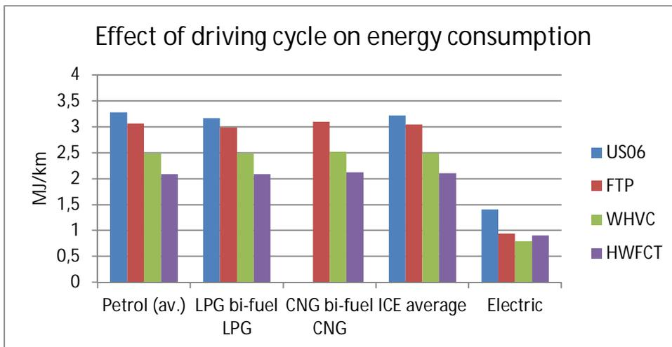
Figure 7.1. The effects of test cycle on energy consumption. Category 1 vans.
