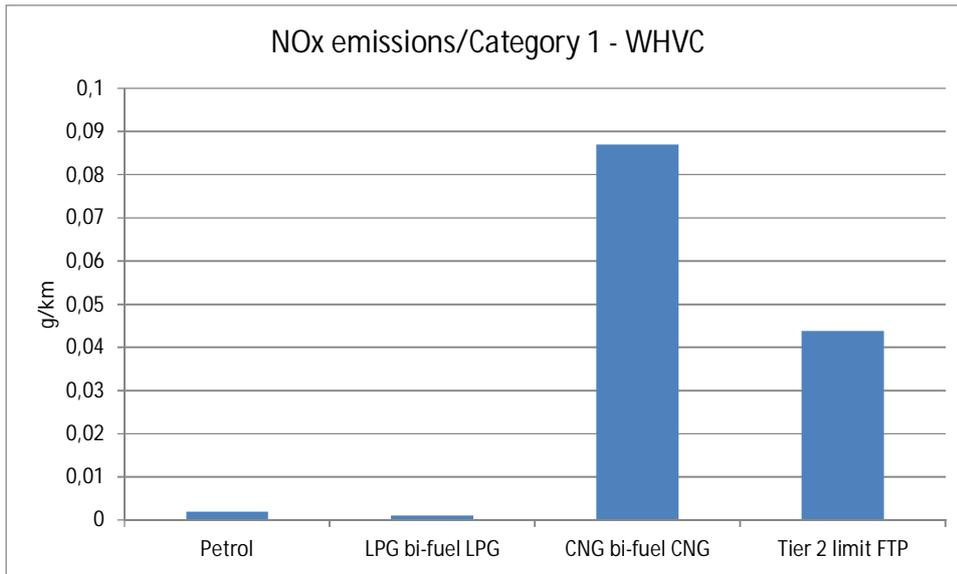
Figure 7.57. NO<sub>x</sub> emissions. North-American Category 1 vehicles. The Tier 2 limit for FTP is shown as a reference.
