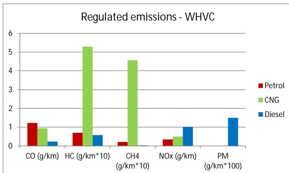
Figure 7.42. Regulated emissions. Euro 4 certified Category 1 pick-ups. PM emissions were not measured for the bi-fuel vehicle.
