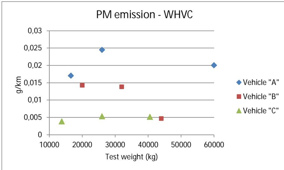
Figure 7.36. Effect of test weight on PM emissions. Euro VI certified Category 3 vehicles.
