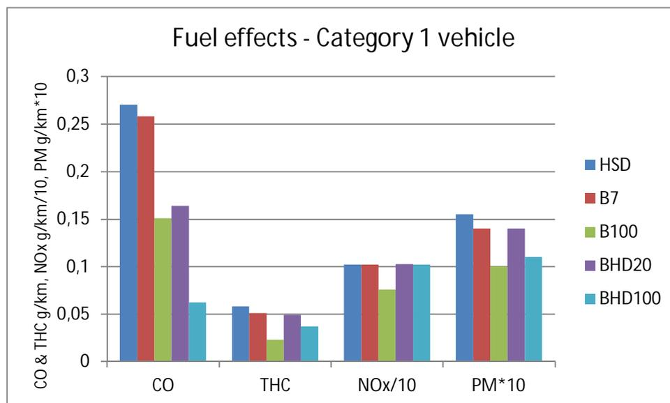
Figure 8.12. Fuel effects on regulated emissions of a Euro 4 certified Category 1 pick-up truck.
