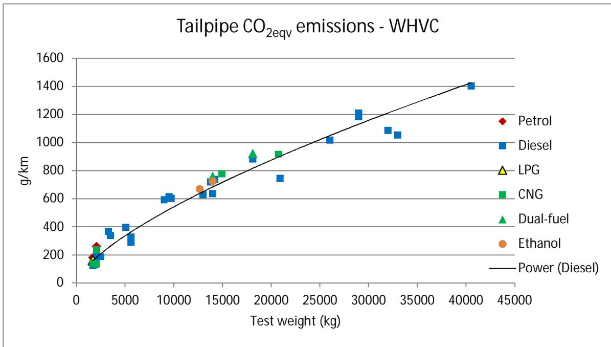
Figure 7.50. CO<sub>2eqv</sub> emissions by fuel.
