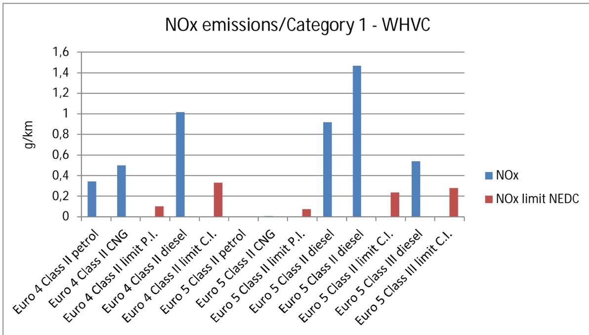
Figure 7.58. NO<sub>x</sub> emissions. Euro certified Category 1 vehicles. The NEDC limit is shown as a reference.
