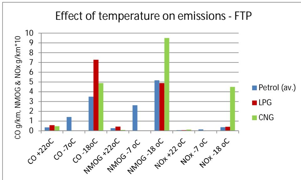
Figure 7.7. The effects of test temperature on emissions. Category 1 vans.
