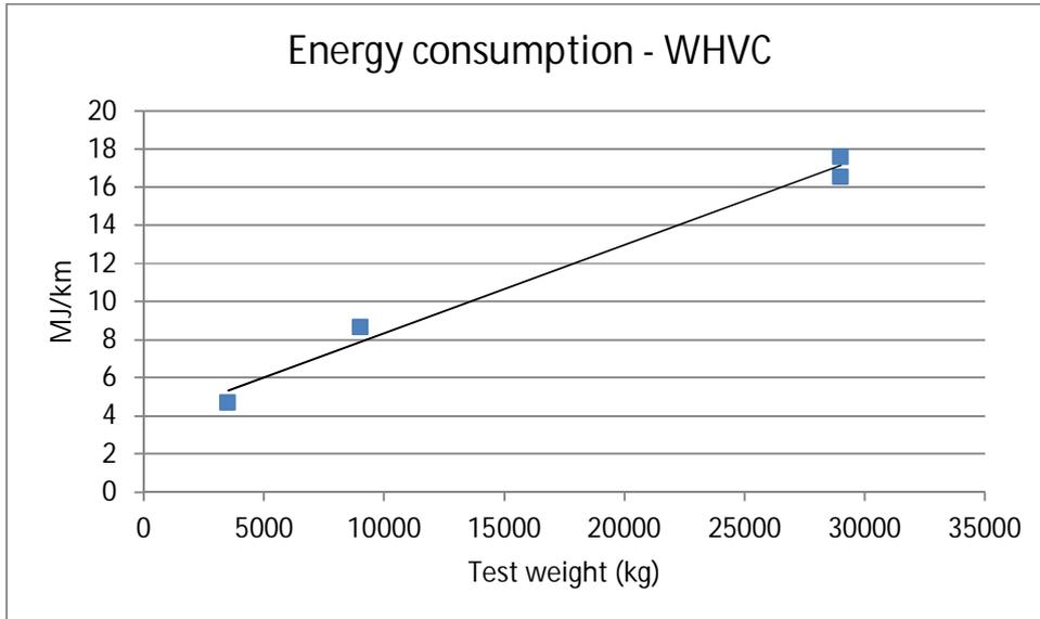
Figure 7.15. Energy consumption vs. test weight.
