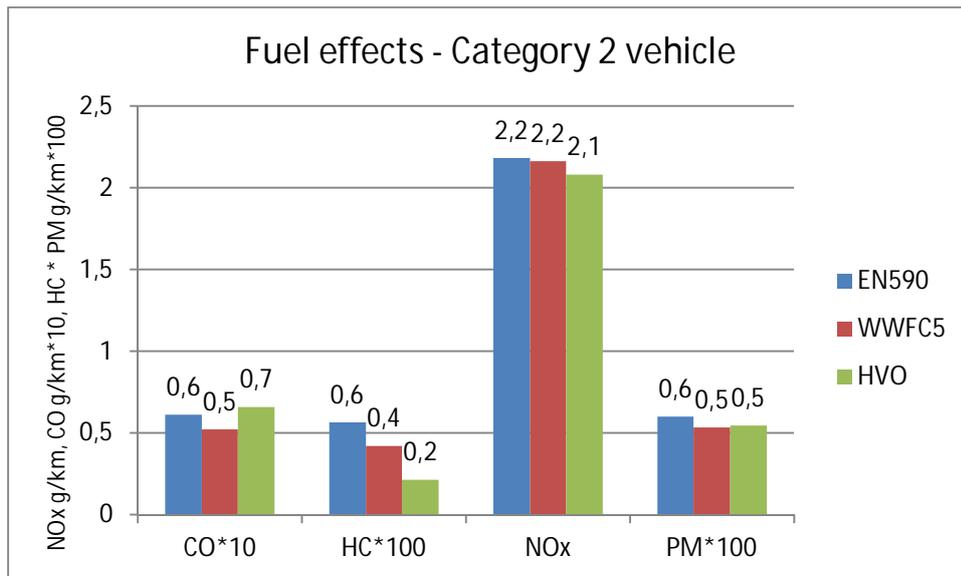
Figure 8.2. Fuel effects on regulated emissions of a Euro V certified Category 2 truck.
