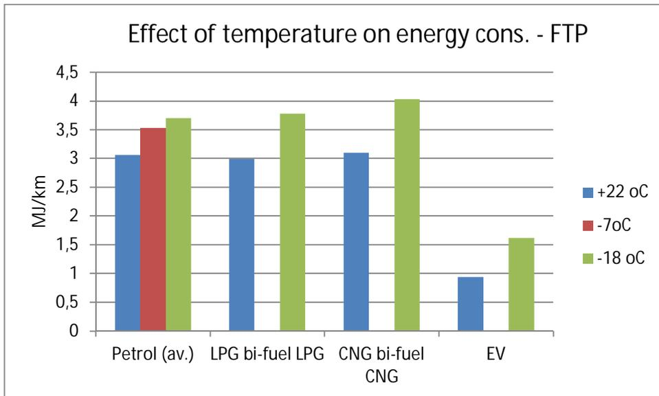
Figure 7.6. The effects of test temperature on energy consumption. Category 1 vans.
