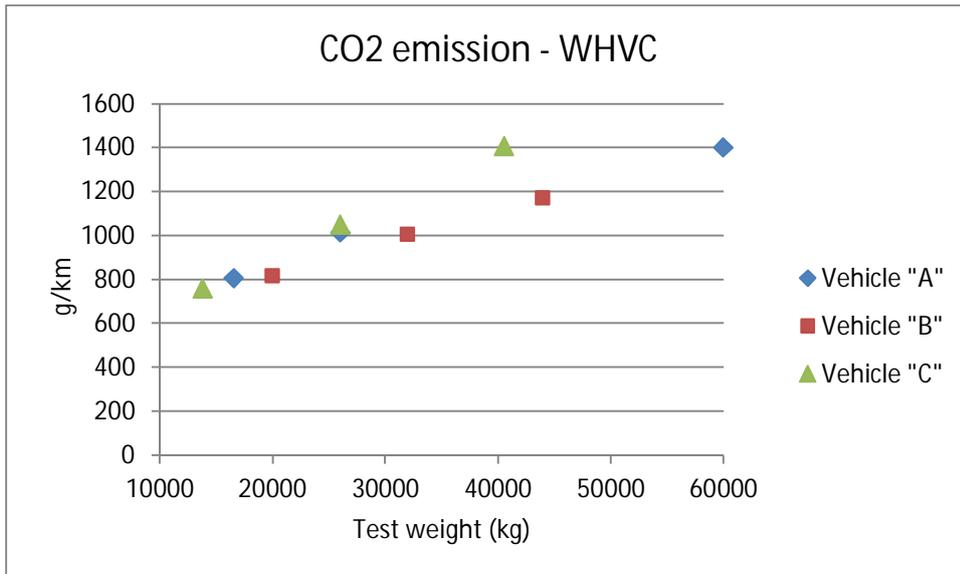
Figure 7.34. Effect of test weight on CO<sub>2</sub> emissions. Euro VI certified Category 3 vehicles.
