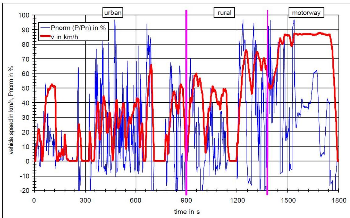
Figure 5.1. The World Harmonised Vehicle Cycle WHVC. (GRPE 2001)
