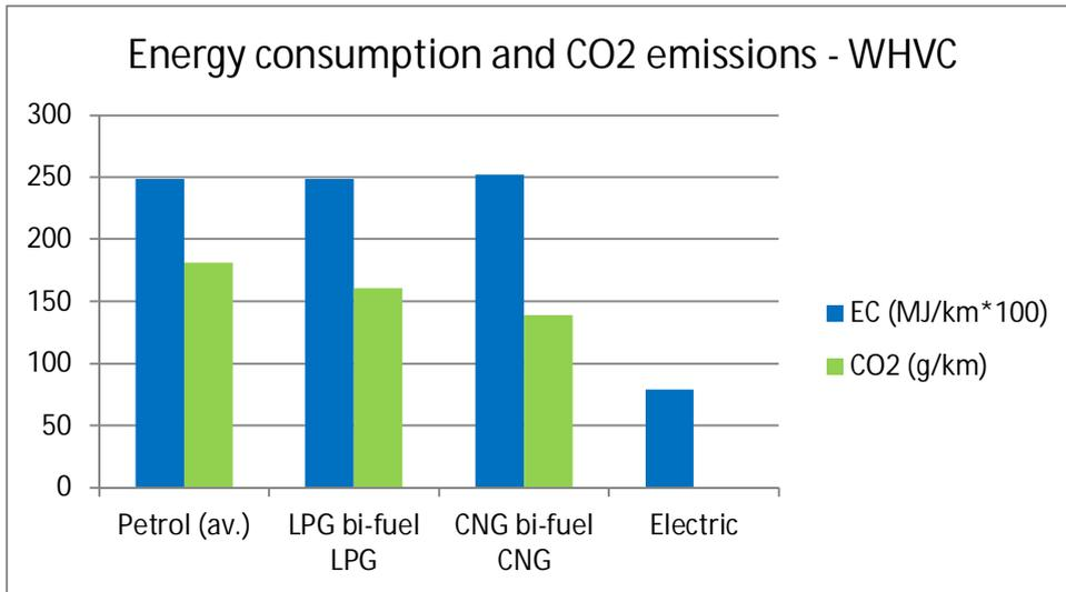
Figure 7.3. Energy consumption and tailpipe CO<sub>2eqv</sub> emissions. Category 1 vans.
