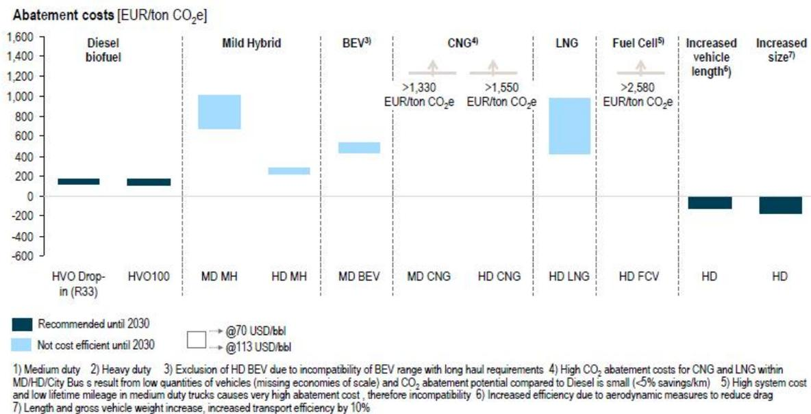
Figure 10.3. CO<sub>2eqv</sub> abatement costs in €/ton for medium- and heavy-duty vehicles. Source Roland Berger.
