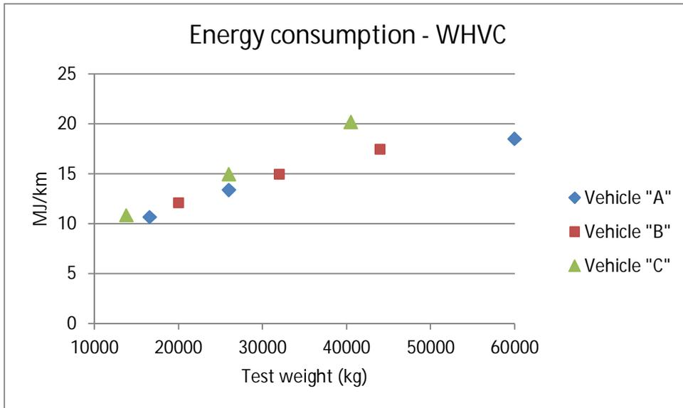
Figure 7.32. Effect of test weight on energy consumption. Euro VI certified Category 3 vehicles.
