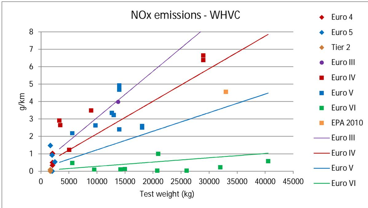
Figure 7.51. NO<sub>x</sub> emissions by emission class.
