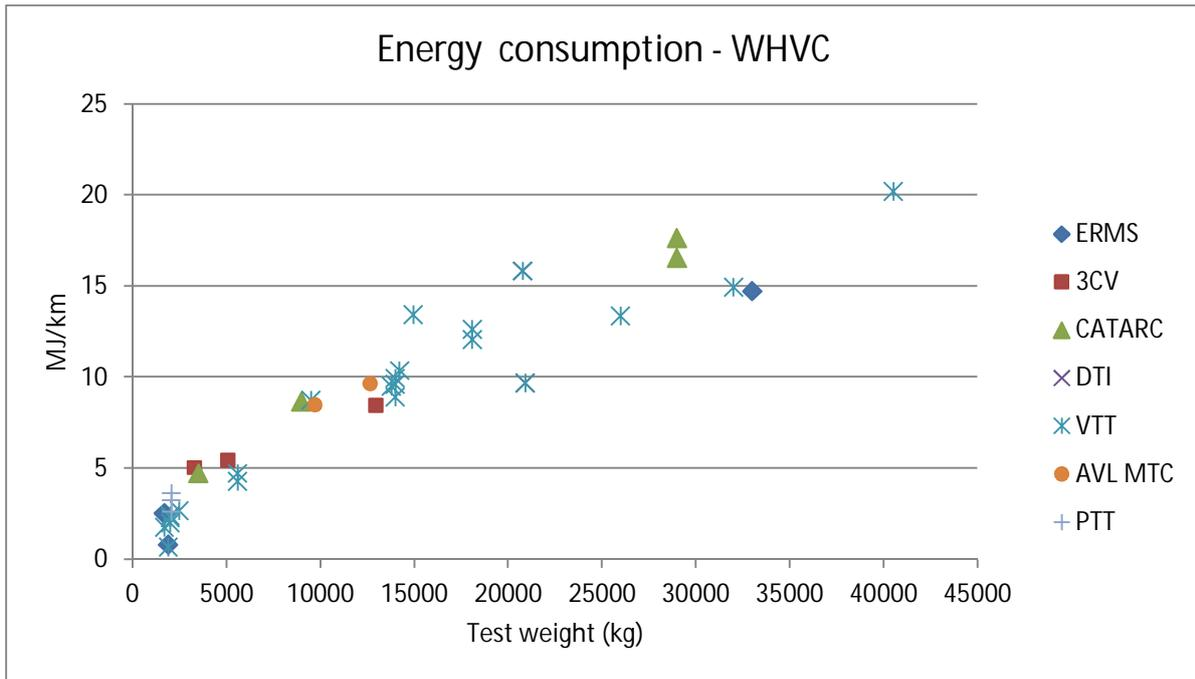
Figure 7.45. Energy consumption by laboratory.
