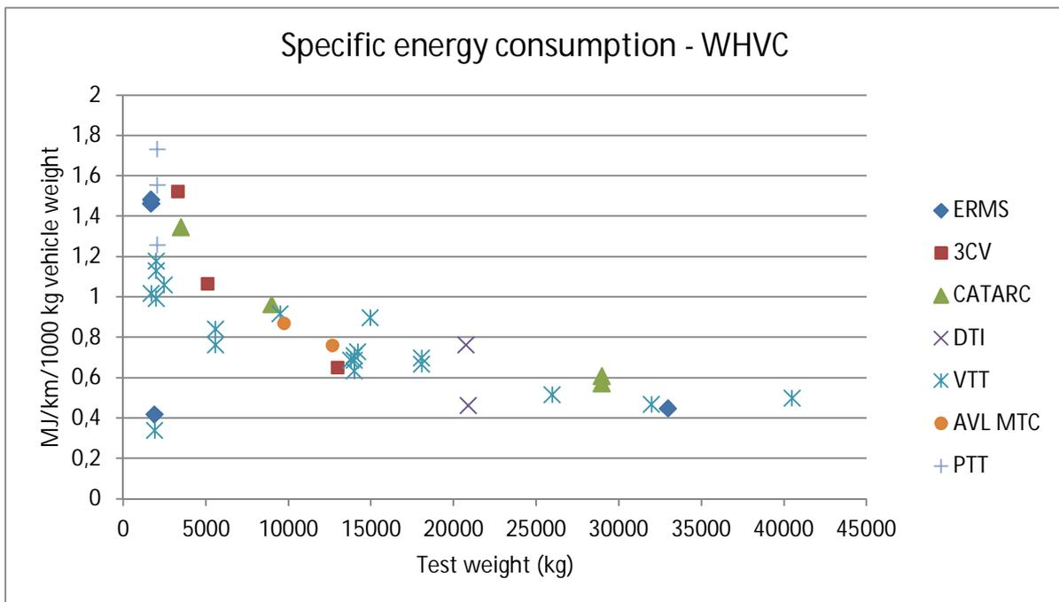
Figure 7.46. Specific energy consumption by laboratory.
