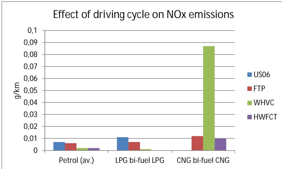
Figure 7.5. The effects of test cycle on NO<sub>x</sub> emissions. Category 1 vans.
