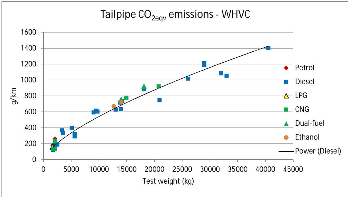
Figure 0.4. CO<sub>2eqv</sub> emissions by fuel.
