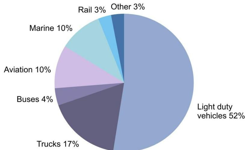
Figure 1.1. Global breakdown of the energy consumption by transportation vehicles (WEF 2011). The 52 % share formed by the light duty vehicles (LDV) contains about 37 %-units of passenger cars and 15 %-units of vans, pick-ups and sport utility vehicles (SUV).
