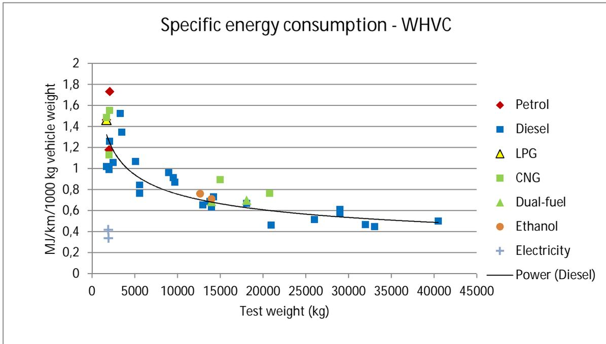
Figure 0.2. Specific energy consumption by fuel.
