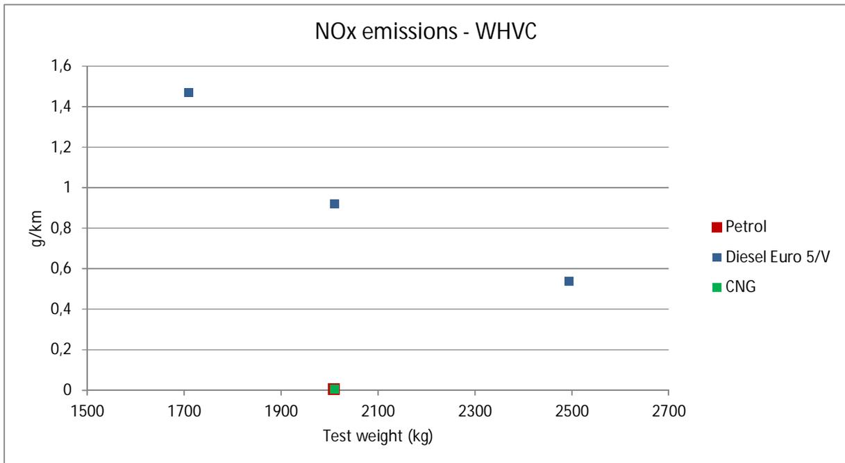
Figure 7.29. NO<sub>x</sub> emissions vs. test weight. Category 1 vehicles (vans).
