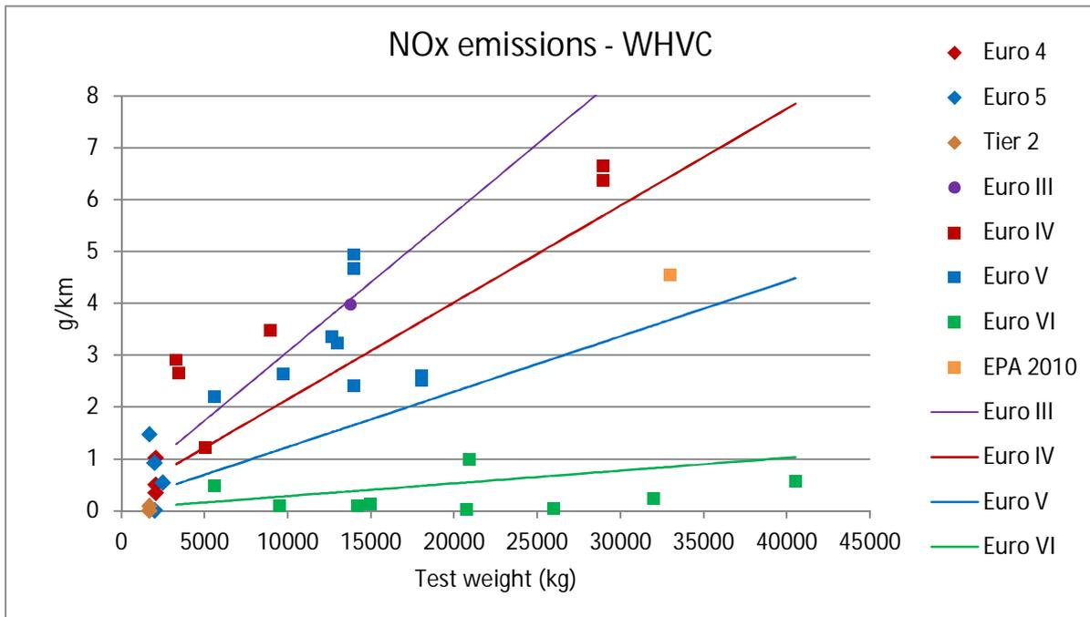
Figure 0.5. NO<sub>x</sub> emissions by emission class.
