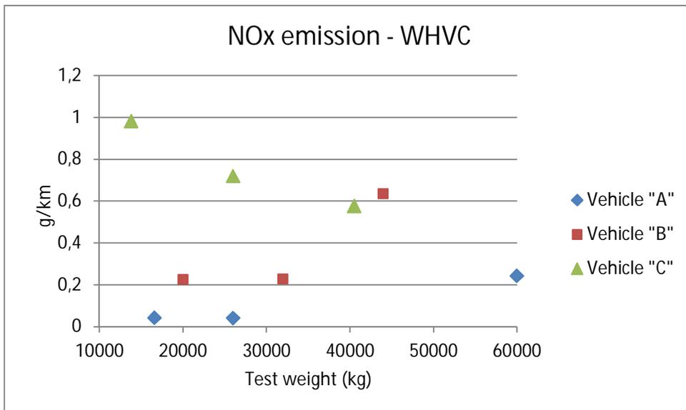
Figure 7.35. Effect of test weight on NO<sub>x</sub> emissions. Euro VI certified Category 3 vehicles.
