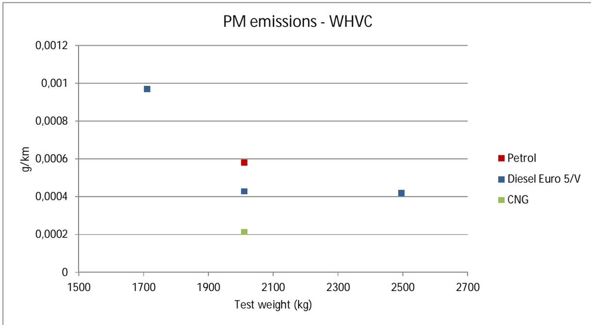
Figure 7.30. PM emissions vs. test weight. Category 1 vehicles (vans).
