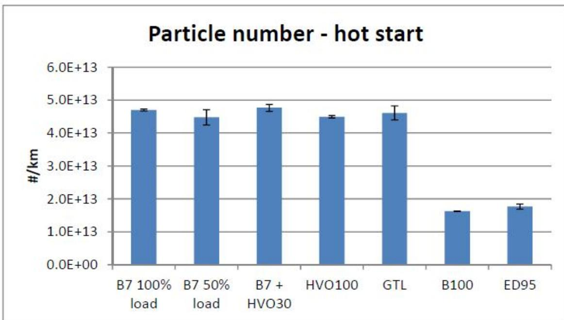
Figure 8.6. Particle number – averaged results from hot start tests.
