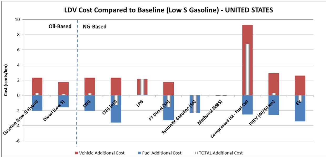
Figure 64: Additional Cost of LDV Natural Gas Pathways in the United States Relative to Low S Gasoline
