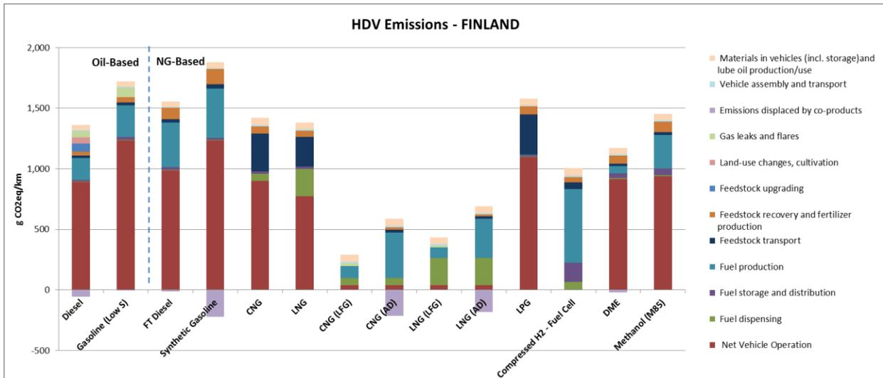
Figure 30: HDV Emissions for Natural Gas Pathways in Finland
