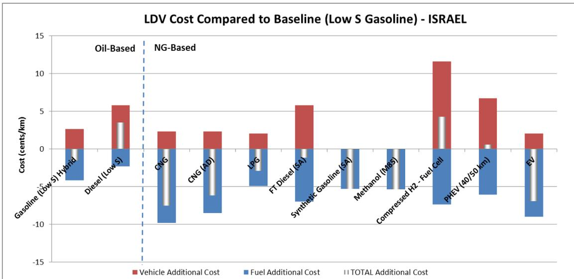
**Figure 62: Additional Cost of LDV Natural Gas Pathways in Israel Relative to Low S Gasoline**
