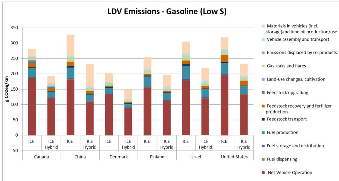
Figure 35: LDV Emissions for Low-S Gasoline
