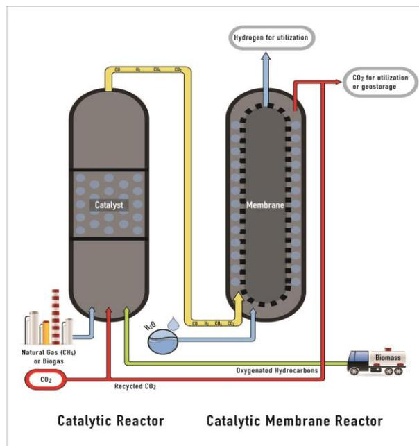
Figure 20: Hydrogen production from natural gas or biomass
