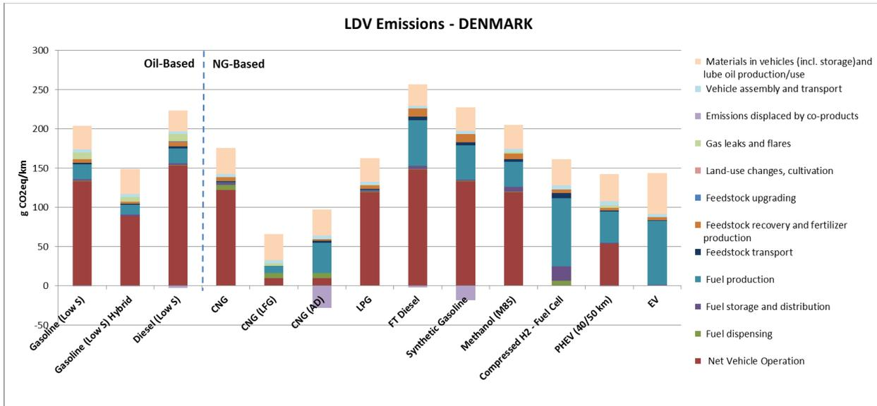
Figure 27: LDV Emissions for Natural Gas Pathways in Denmark
