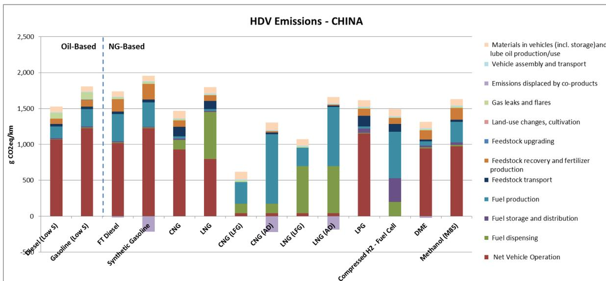
Figure 26: HDV Emissions for Natural Gas Pathways in China
