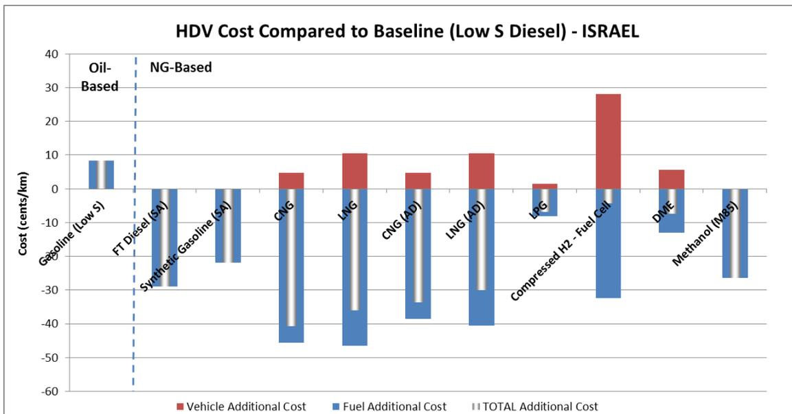
**Figure 63: Additional Cost of HDV Natural Gas Pathways in Israel Relative to Low S Diesel**
