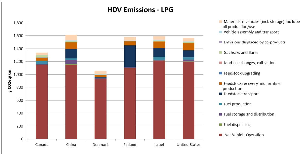
Figure 44: HDV Emissions for LPG
