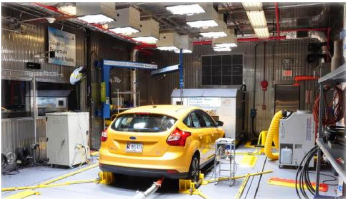
Figure 15: Dynamometer test cell at the Advanced Powertrain Research Facility of ANL.
