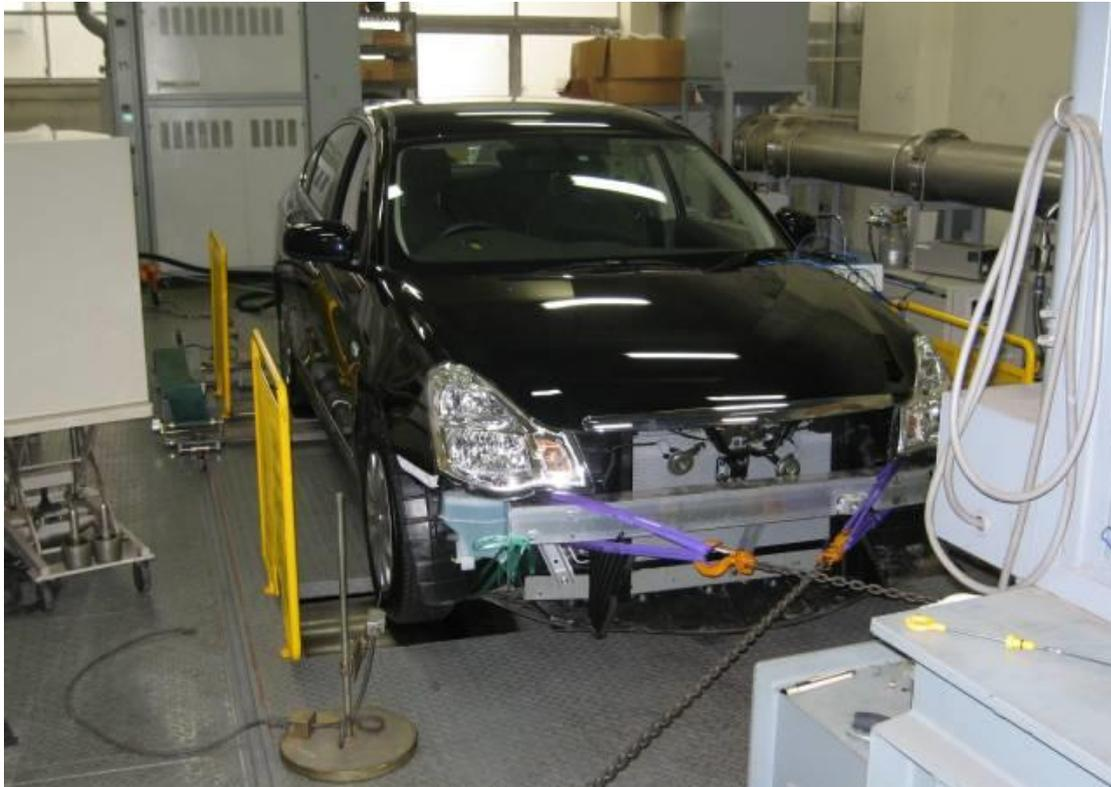
Figure 4: Exhaust emissions test cell at National Traffic Safety and Environment Laboratory (NTSEL), Japan.
