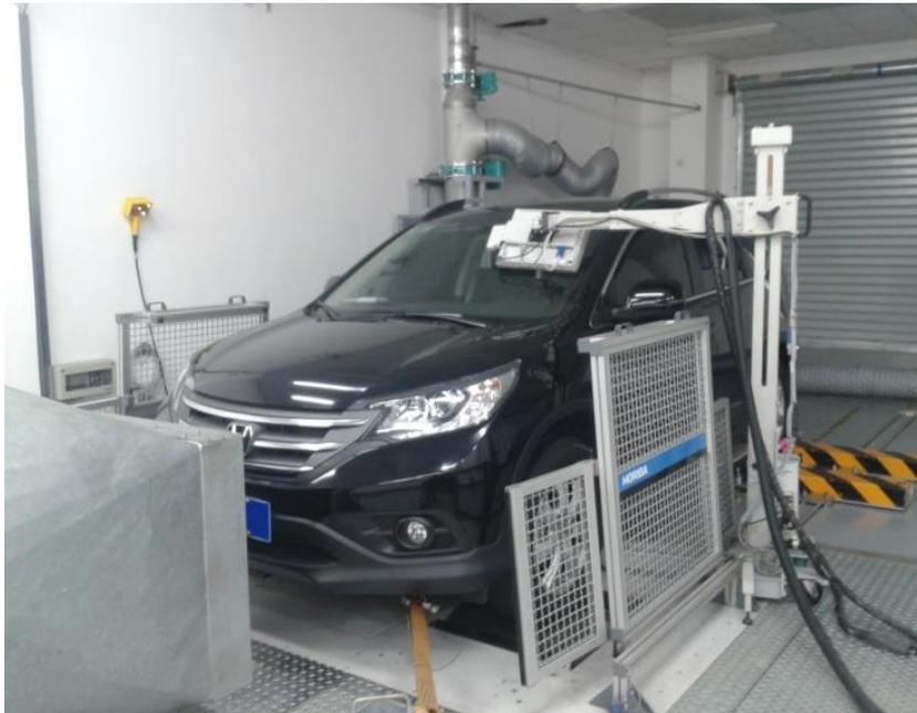
*Figure 8: Light duty vehicle emissions test cell at CATARC, China.*
