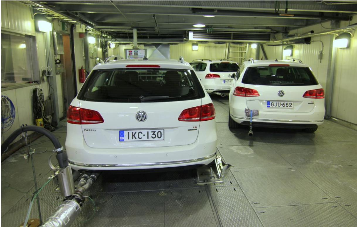
Figure 10: Test cell at VTT is large enough to be used to soak/precondition and test up to three cars simultaneously during a single 8-hour working day.
