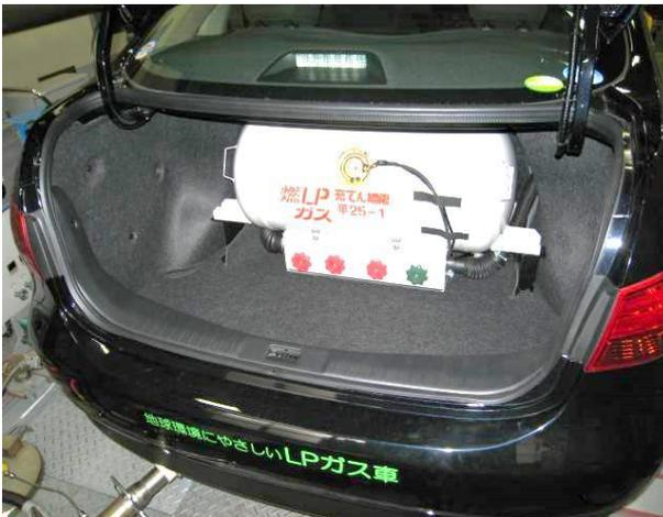
Figure 3: LPG-tank of a converted Nissan Bluebird Sylphy (G11-model).
