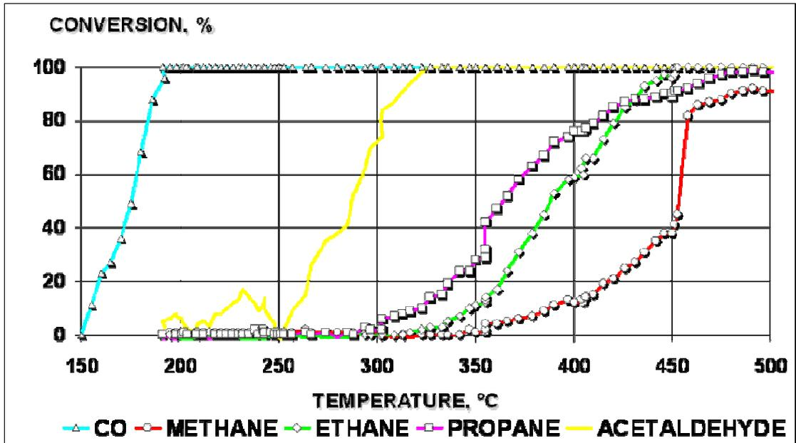
Figure 3. Conversion rate vs. exhaust temperature (Source: Kemira)
