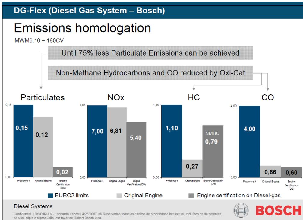
Figure 11. Emission results from Bosch Dual Fuel system eDG-Flex (Source: Bosch Brazil)
