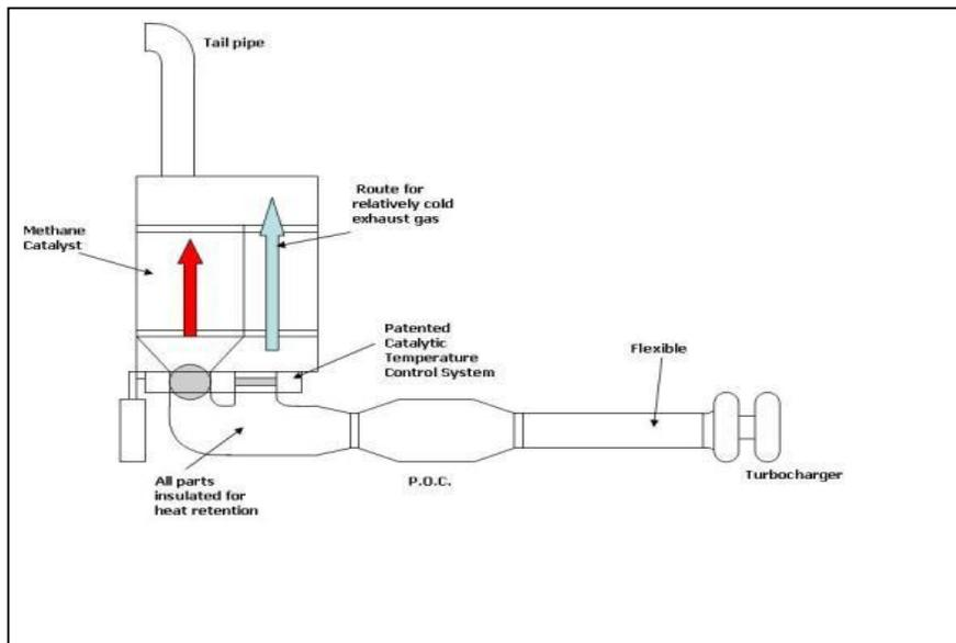
**Figure 9.** Hardstaff patented catalytic temperature control
