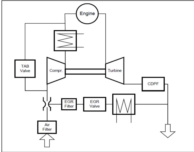
**Figure 6.** Basic lay-out of PACCOLD-EGR system
