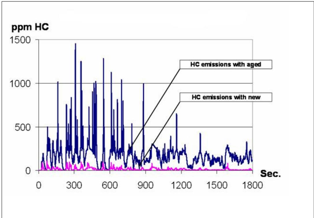
**Figure 4.** THC emissions with a lean burn engine in the European Transient Cycle (ETC) with a new and a catalyst damaged from misfire. (after 10 executive cycles)
