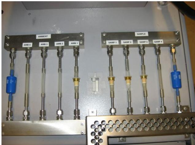
Figure 28: Horiba NMOG sample cart system (VCC).
