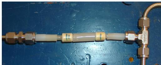
Figure 21: DNPH cartridges used for aldehyde sampling, two in series.
