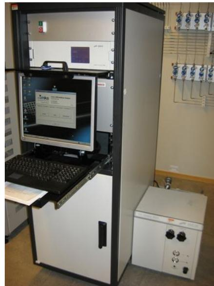
Figure 25: The FTIR measures ethanol and aldehydes concentrations online.
