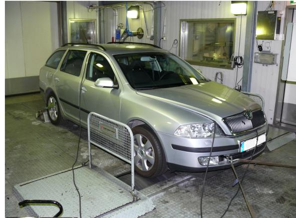
Figure 29: The test vehicle on the chassis dynamometer.
