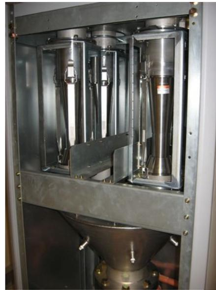
Figure 23: Critical flow venturi.
