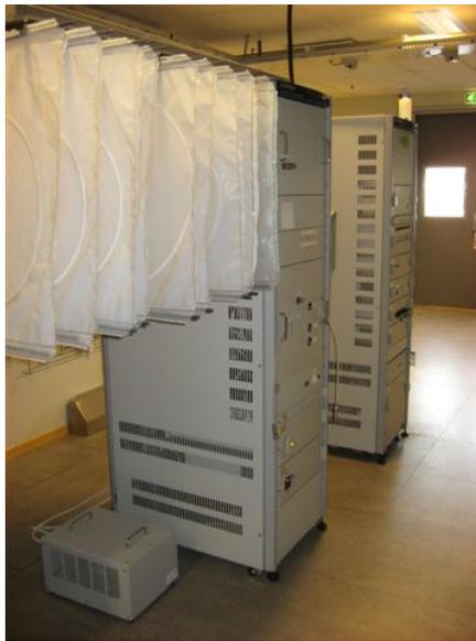
Figure 22: Horiba CVS-7200SLE sampling system.
