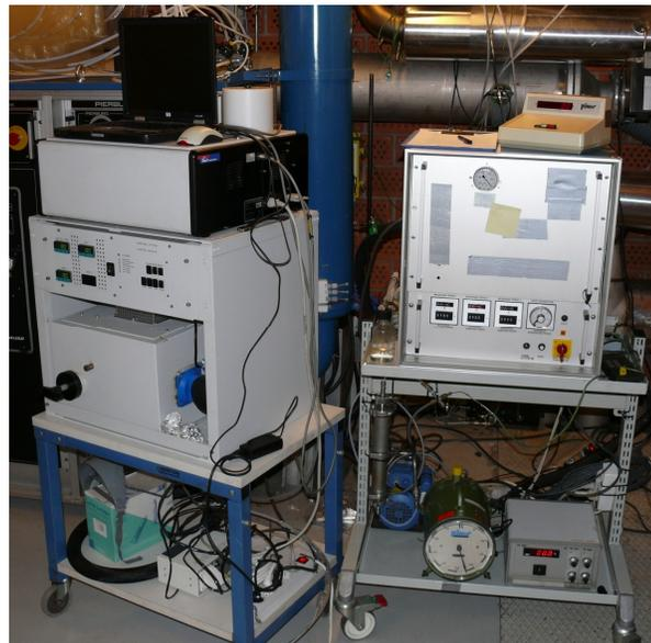
Figure 32: The FTIR (left) and the DNPH cartridges sampling system (right) at VTT.
