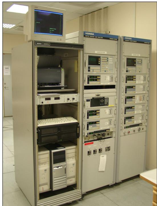
Figure 17: Horiba MEXA measurement system.
