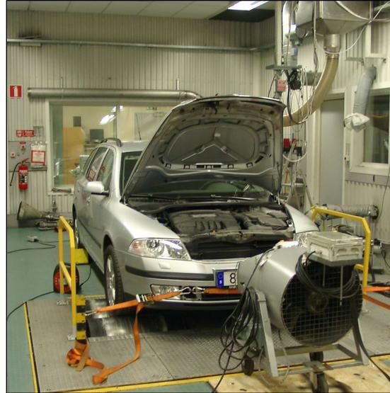
Figure 16: The test vehicle on the chassis dynamometer.
