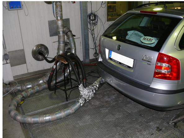
Figure 31: Sampling from exhaust pipe, FTIR and AMA.
