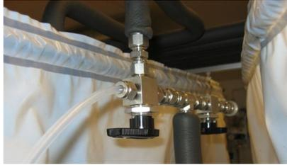
Figure 26: Switch between bag analysis and INNOVA.
