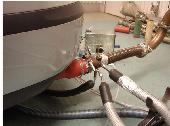
Figure 19: Sampling of raw exhaust emissions from the tailpipe.
