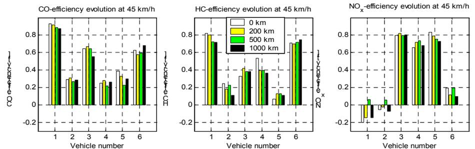
Figure 3: Trend of catalyst efficiencies at 45 km/h over mileage.
