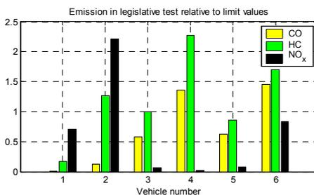
Figure 1: CO, HC and NO<sub>x</sub> emissions of ECE40m test, relative to legislation level.
