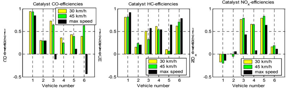
Figure 2: Catalyst efficiencies at different constant load points for new vehicles.
