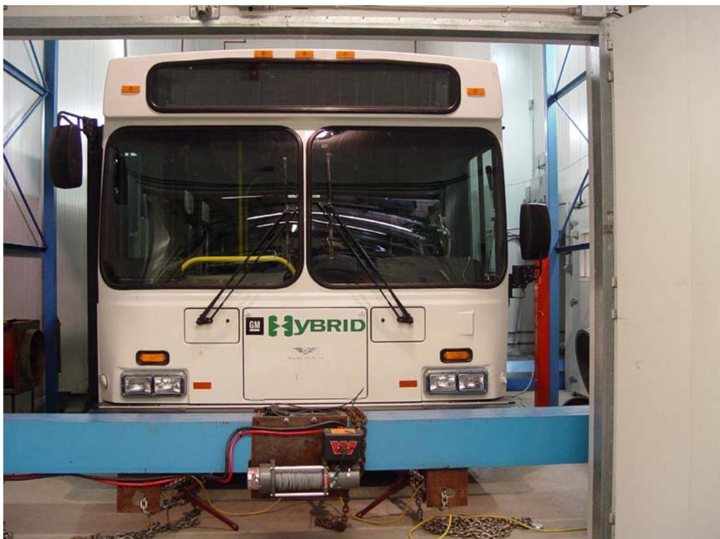
*Figure 4.6. A hybrid bus on Environment Canada's chassis dynamometer.*
