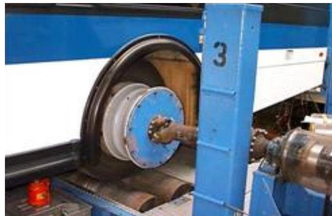
*Figure 4.8. Hub adapters connect vehicle's drive axle directly to the power absorber unit.*
