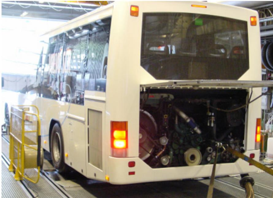
*Figure 4.5. Emission testing on VTT's chassis dynamometer.*
