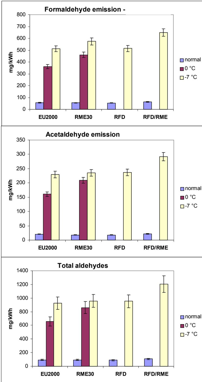
Figure 12. Aldehyde emissions with the medium-duty engine.
