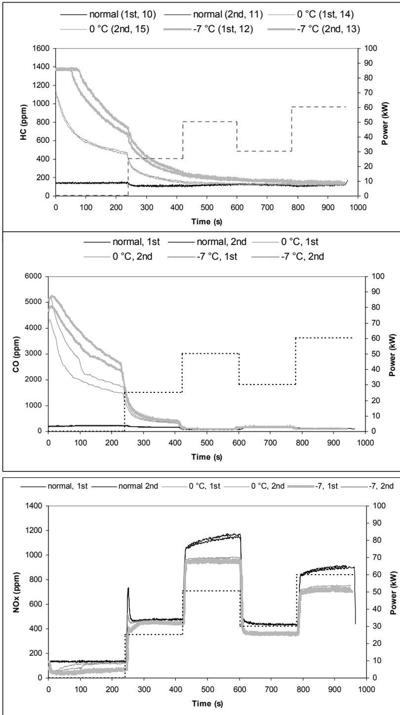
Figure 10. CO, HC and NO<sub>x</sub> concentrations, medium-duty engine.
