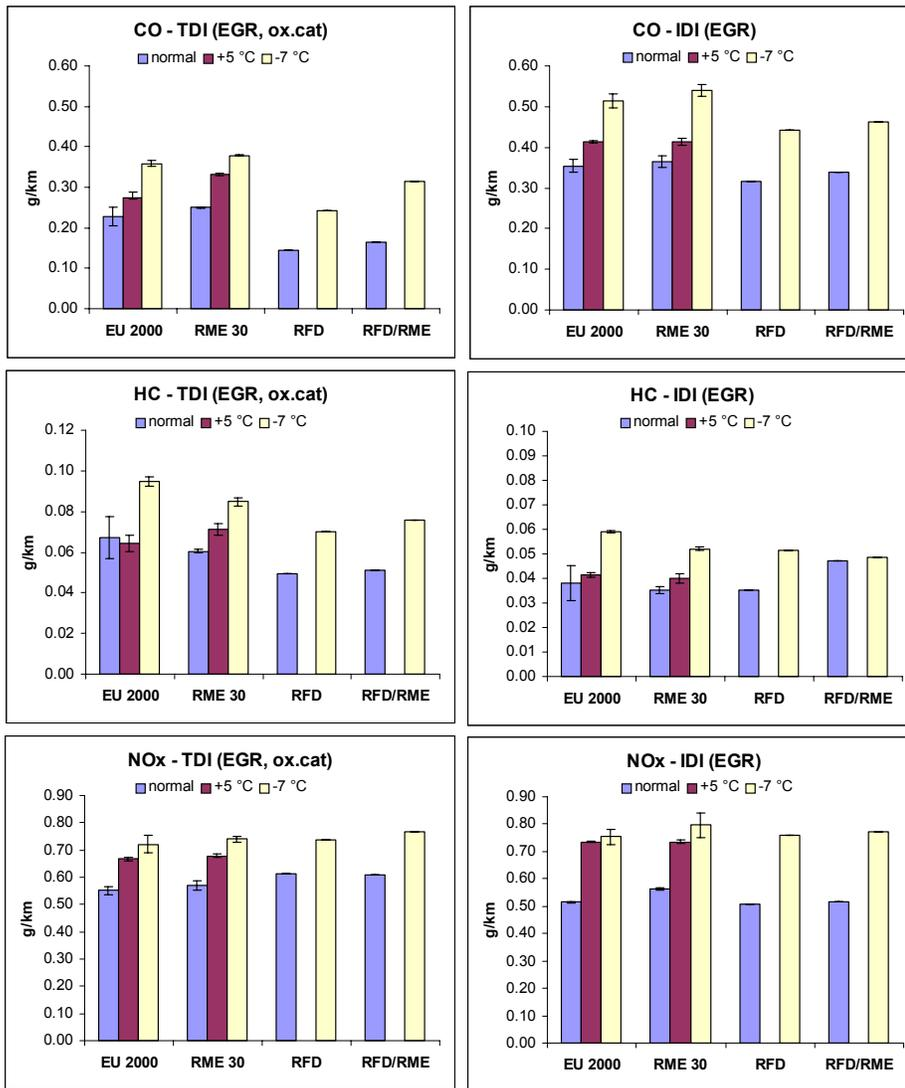
Figure 39. CO, HC and NO<sub>x</sub> emissions over the European test cycle with the TDI and IDI cars.
