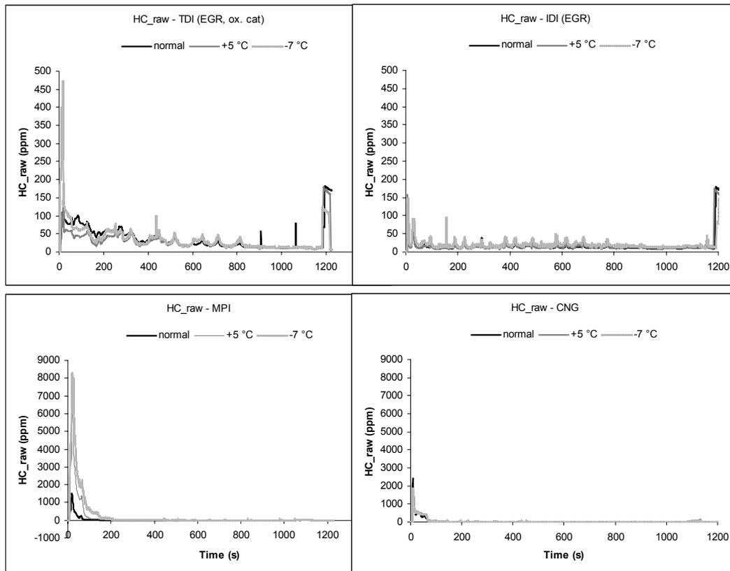
Figure 25. Continuous raw exhaust gas concentrations of CO, HC and NO<sub>x</sub> during the European test cycle.
