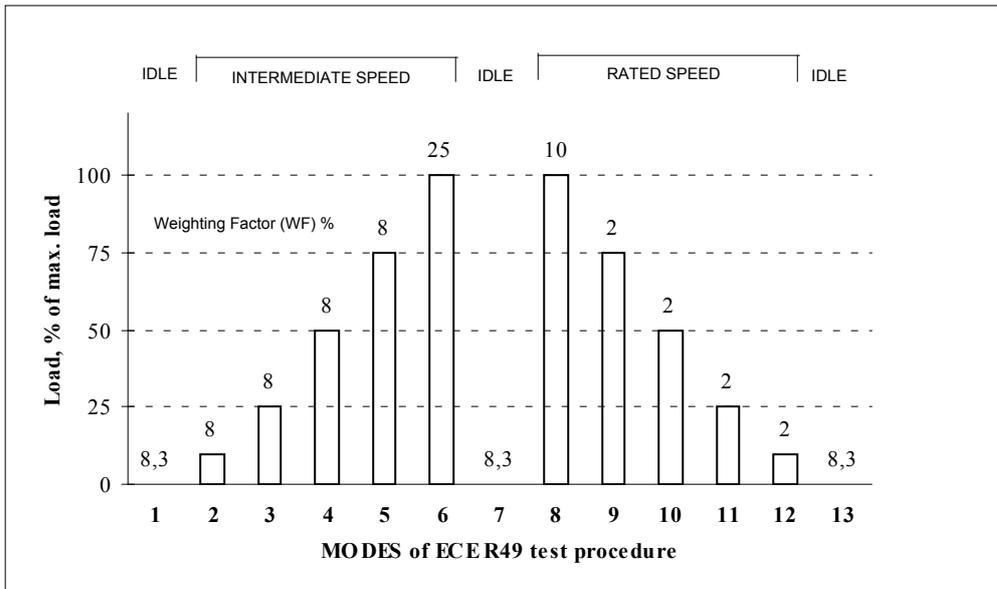
Figure 3. Test sequence of the ECE R49 13-mode test cycle
