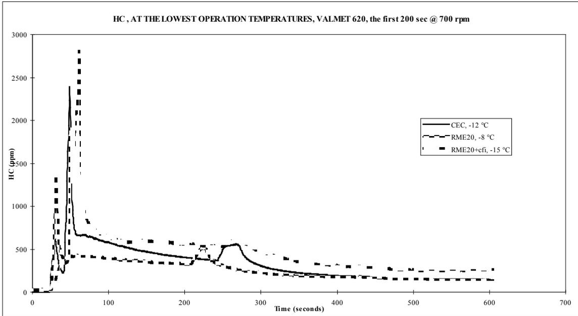
Figure 33. HC concentrations in the cold start test, Valmet 620.
