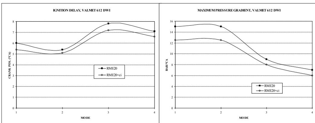
Figure 18. The ignition delay and maximum pressure gradient at different loads of ECE R49 test with VALMET 612 DWI. The ignition delay is shorter, when the cetane improver additive is used.
