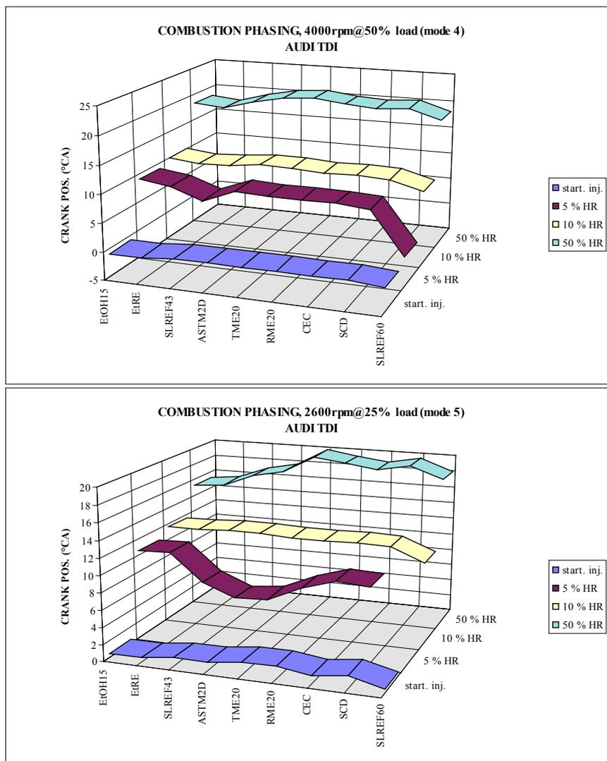
Figure 24. Combustion parameters of the test fuels with Audi 1.9 TDI vehicle at loads 4000 rpm / 50 % load (mode 1) and 2600 rpm / 25 % load (mode 5). The test fuels are presented in increasing order of cetane number.
