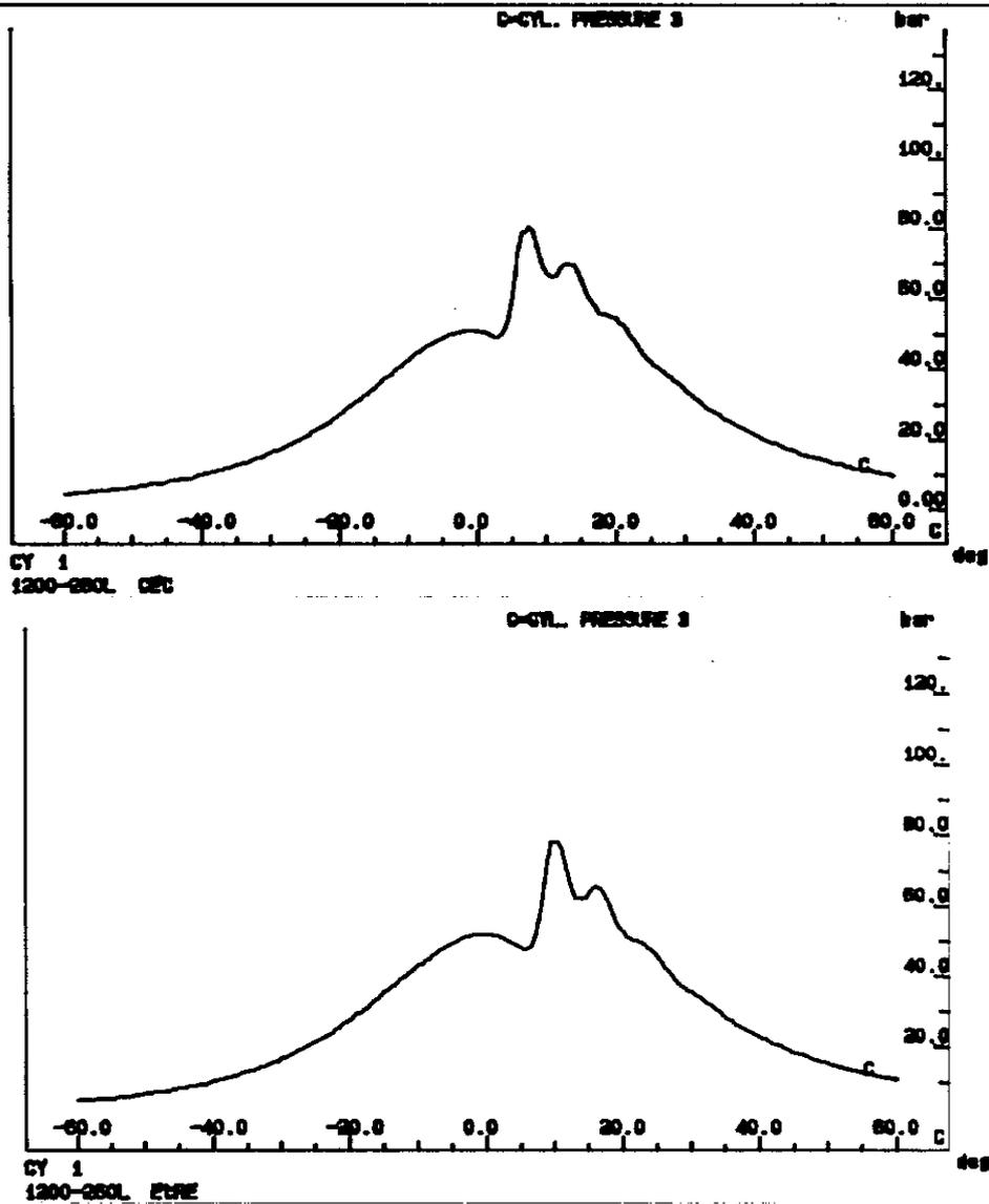
*Figure 14. Cylinder pressure curves for the VALMET 612 DWI engine at intermediate speed, 50% load with CEC and EtRE fuels.*
