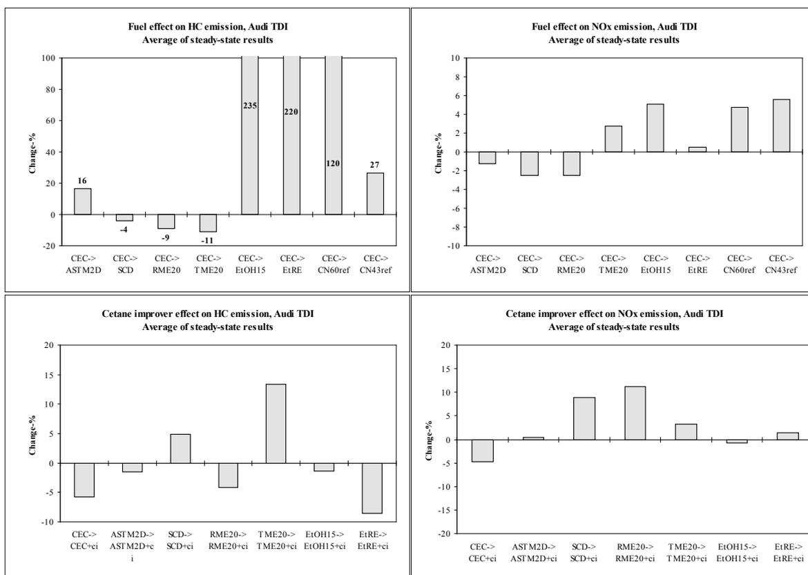
Figure 23. HC and NO<sub>x</sub>-emission changes in Audi 1.9 TDI steady-state tests. Changes of less than 10% for HC are insignificant.
