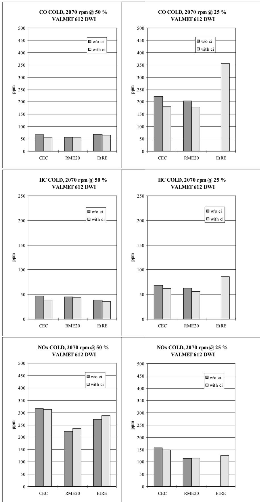
Figure 41. Exhaust concentrations with the VALMET 612 DWI engine (cold engine under load).
