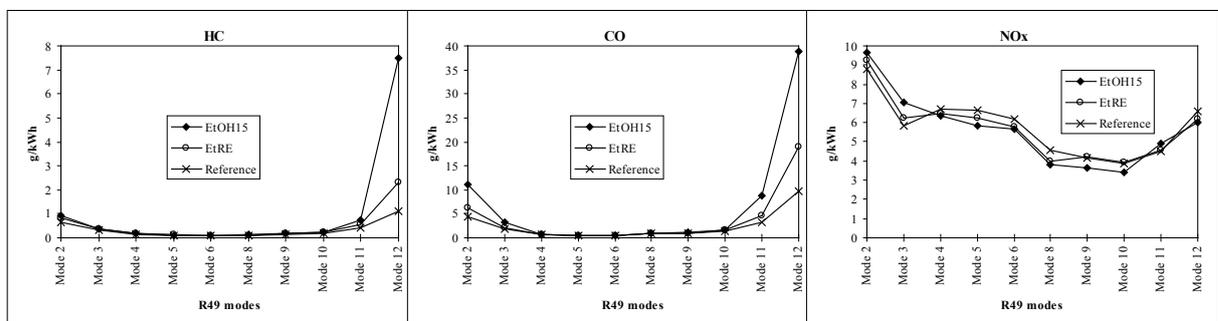
Figure 7. Comparison of the ethanol blends and the reference fuel in different modes of ECE R49. Modes 5, 6, 8, and 9 are high-loads (75 - 100% of maximum) and the others low loads (10 - 50% of maximum load).
