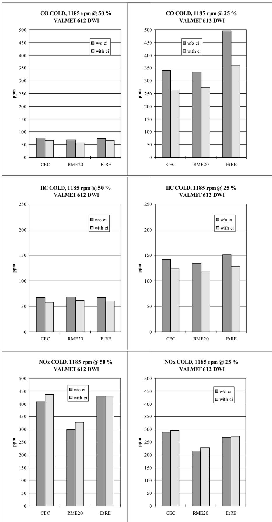
Figure 40. Exhaust concentrations with the VALMET 612 DWI engine (cold engine under load).
