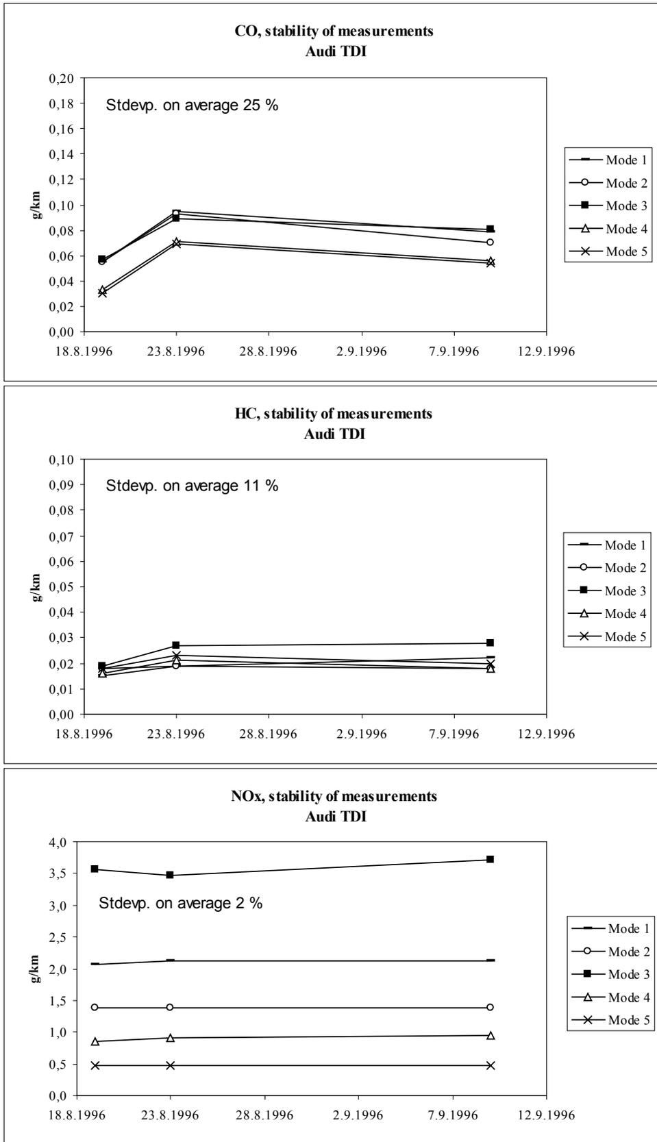
Figure 21. Stability of the measuring system over the testing period, steady-state tests with Audi 1.9 TDI.
