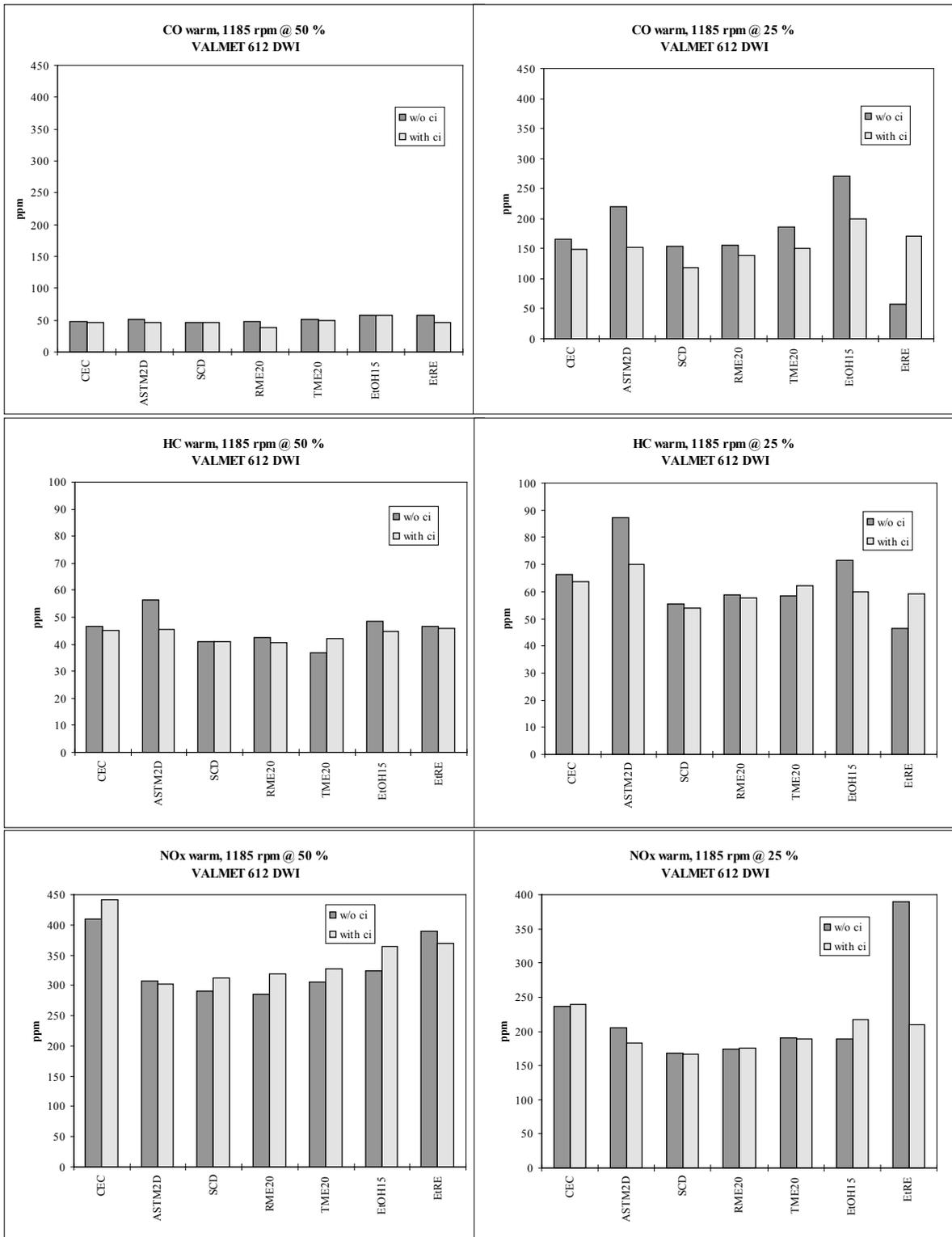
Figure 15. CO, HC and NO<sub>x</sub> concentrations at intermediate speed, 50 and 25% loads with the Valmet 612 DWI engine.
