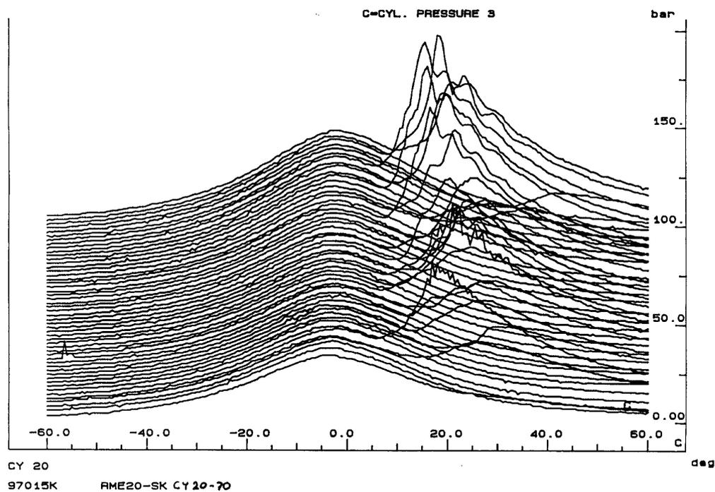
Figure 35. Cylinder pressure curves for the CEC and RME20+ci fuels during some 50 working cycles after the start of the engine at  $-6^{\circ}\text{C}$ .
