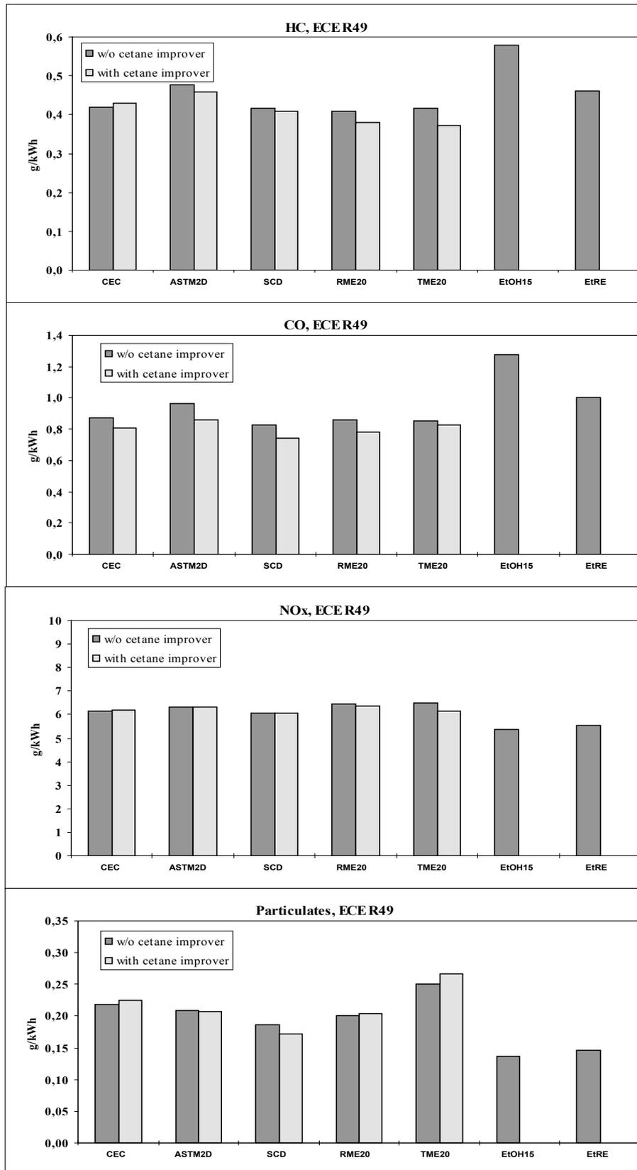
Figure 8. The regulated emissions of the heavy-duty VOLVO engine according to the ECE R49 test procedure.
