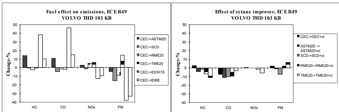
Figure 6. Changes in emissions with VOLVO THD 103 KB according to ECE R49 test procedure. Changes of gaseous emissions lower than 5% and particulates lower than 10% are insignificant.
