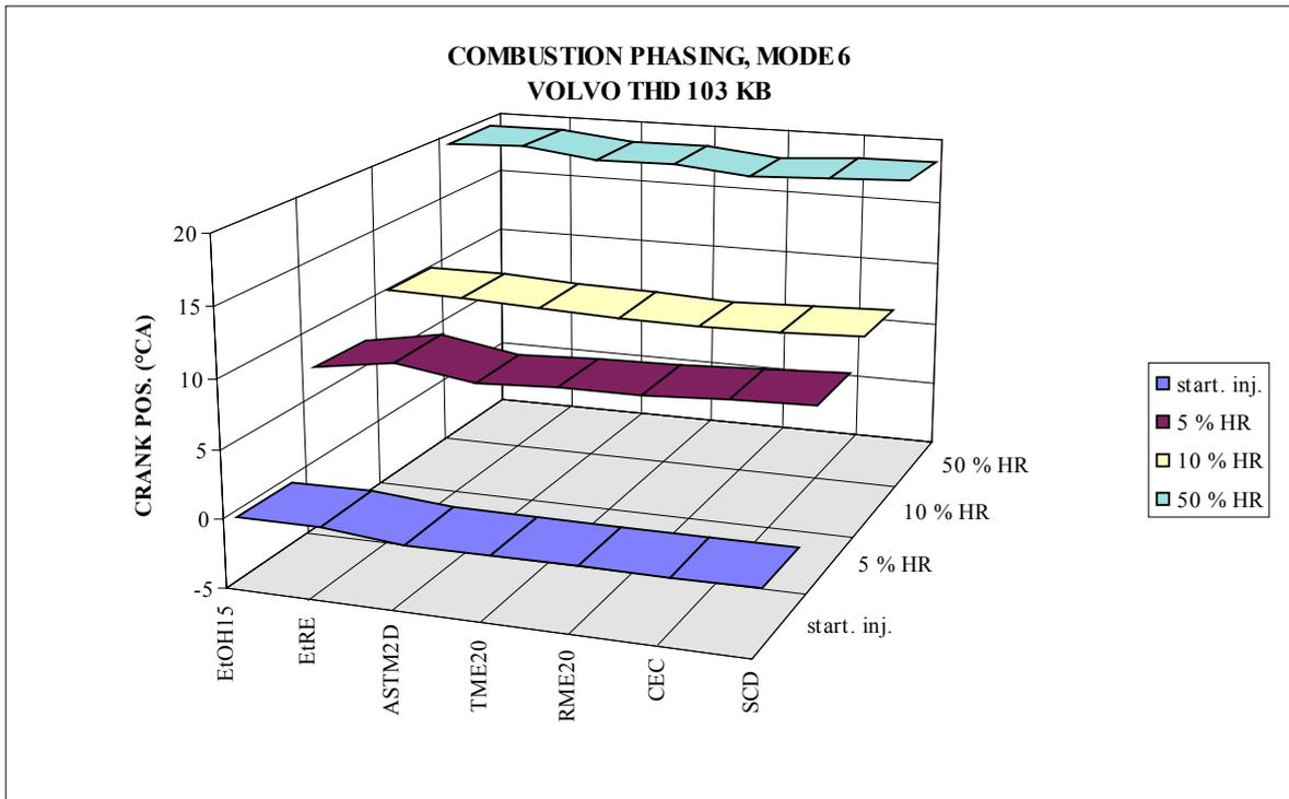
Figure 11. Start of injection, 5, 10 and 50% heat release of the test fuels with VOLVO THD 103 KB engine at high load mode 6 and low load mode 12 of ECE R49 test. The test fuels are presented in increasing order of cetane number.
