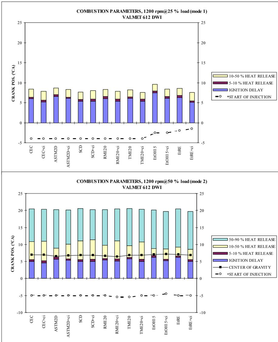
Figure 17. Combustion parameters at intermediate speed 25 and 50% loads for the VALMET 612 DWI engine. The ignition delay is longest for the low cetane fuels.
