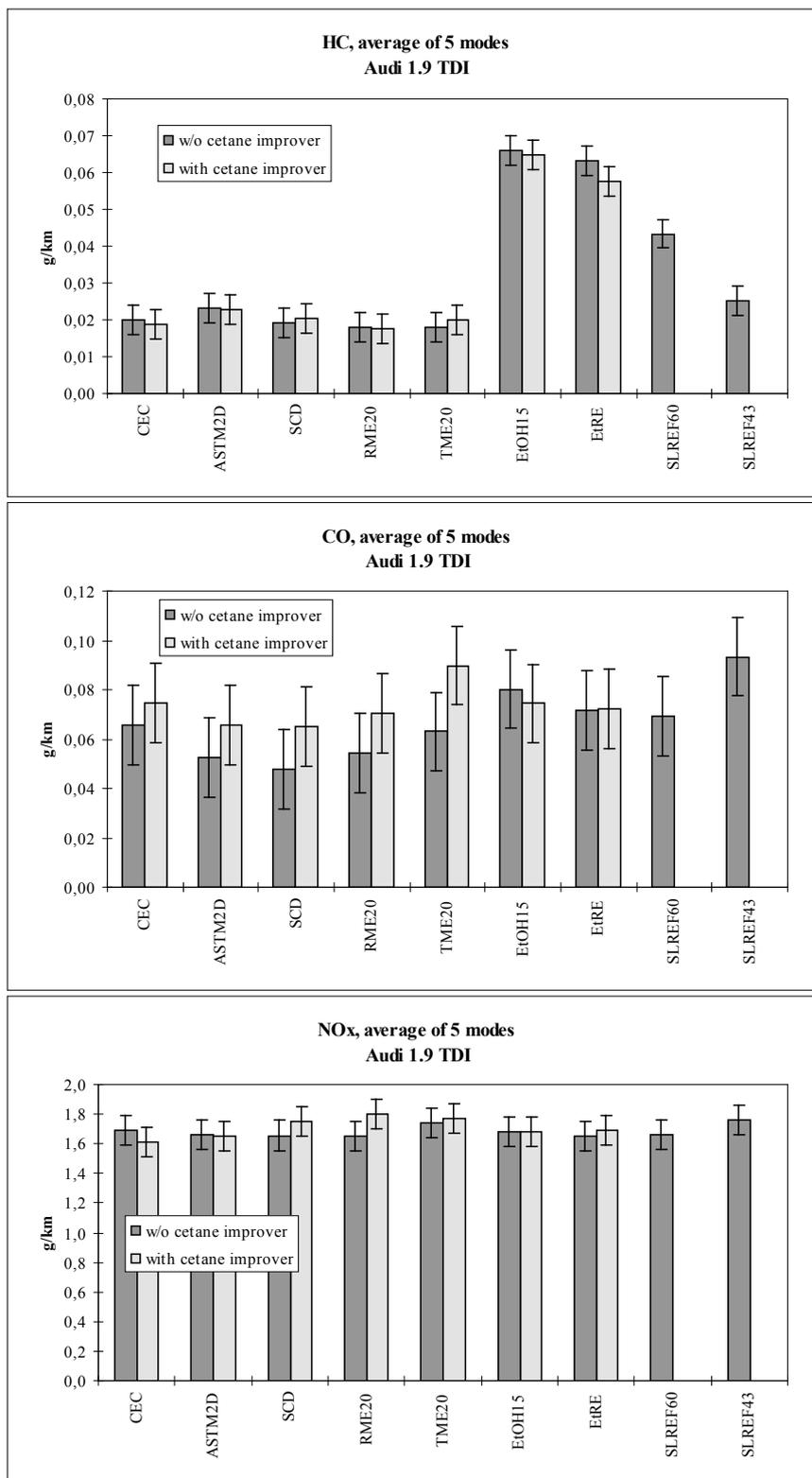
Figure 22. The regulated emissions from Audi 1.9 TDI on average for 5 steady-state loads. The error bars represent standard deviations with the CEC fuel measured three times during the testing period.
