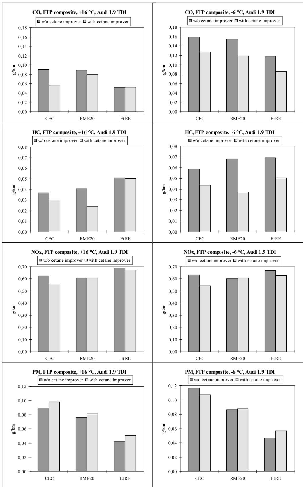
Figure 42. FTP results with Audi 1.9 TDI at +16 and -6 °C temperatures.
