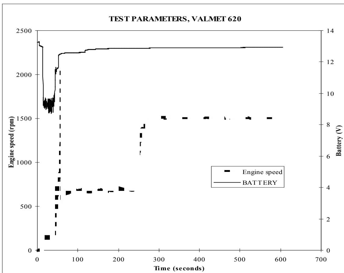
*Figure 31. Engine speed and battery charge during the cold start test.*
