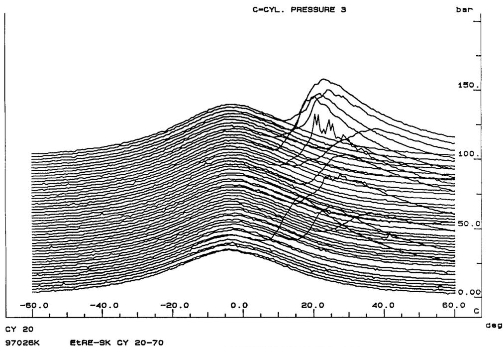
Figure 36. Cylinder pressure curves for the EtRE and EtRE+ci fuels during some 50 working cycles after the start of the engine at  $-6^{\circ}\text{C}$ .
