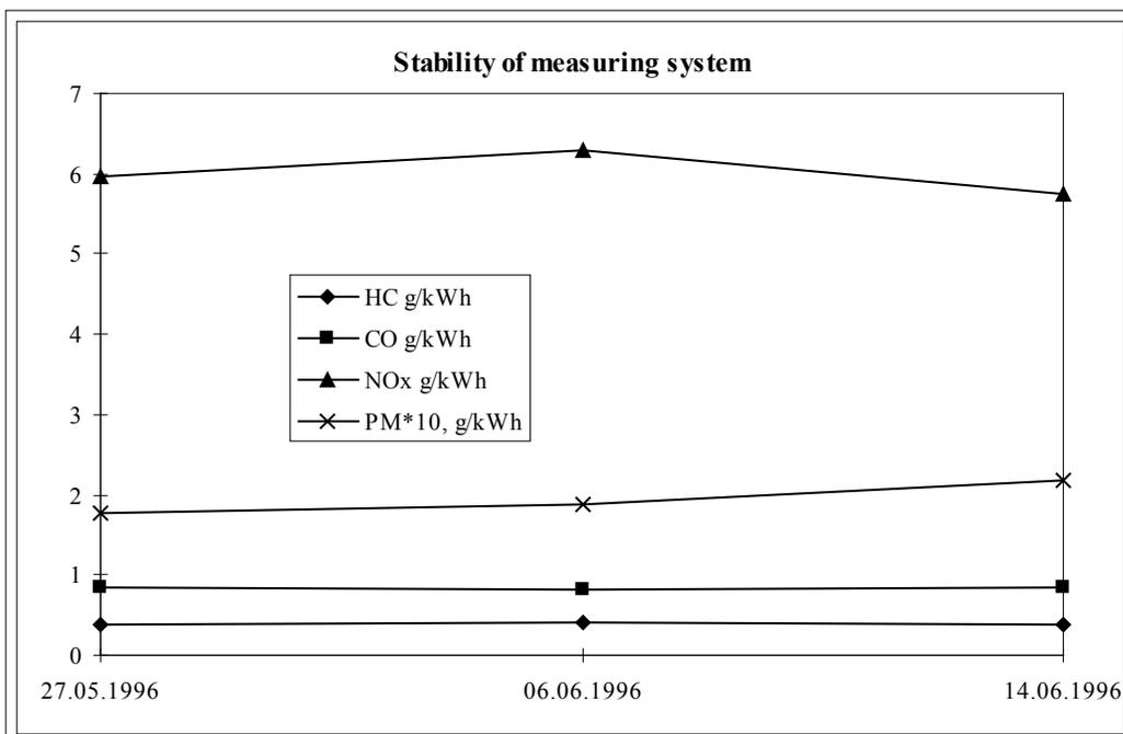
Figure 5. Stability of measuring system, VOLVO THD 103 KB with ECE R49 test procedure.
