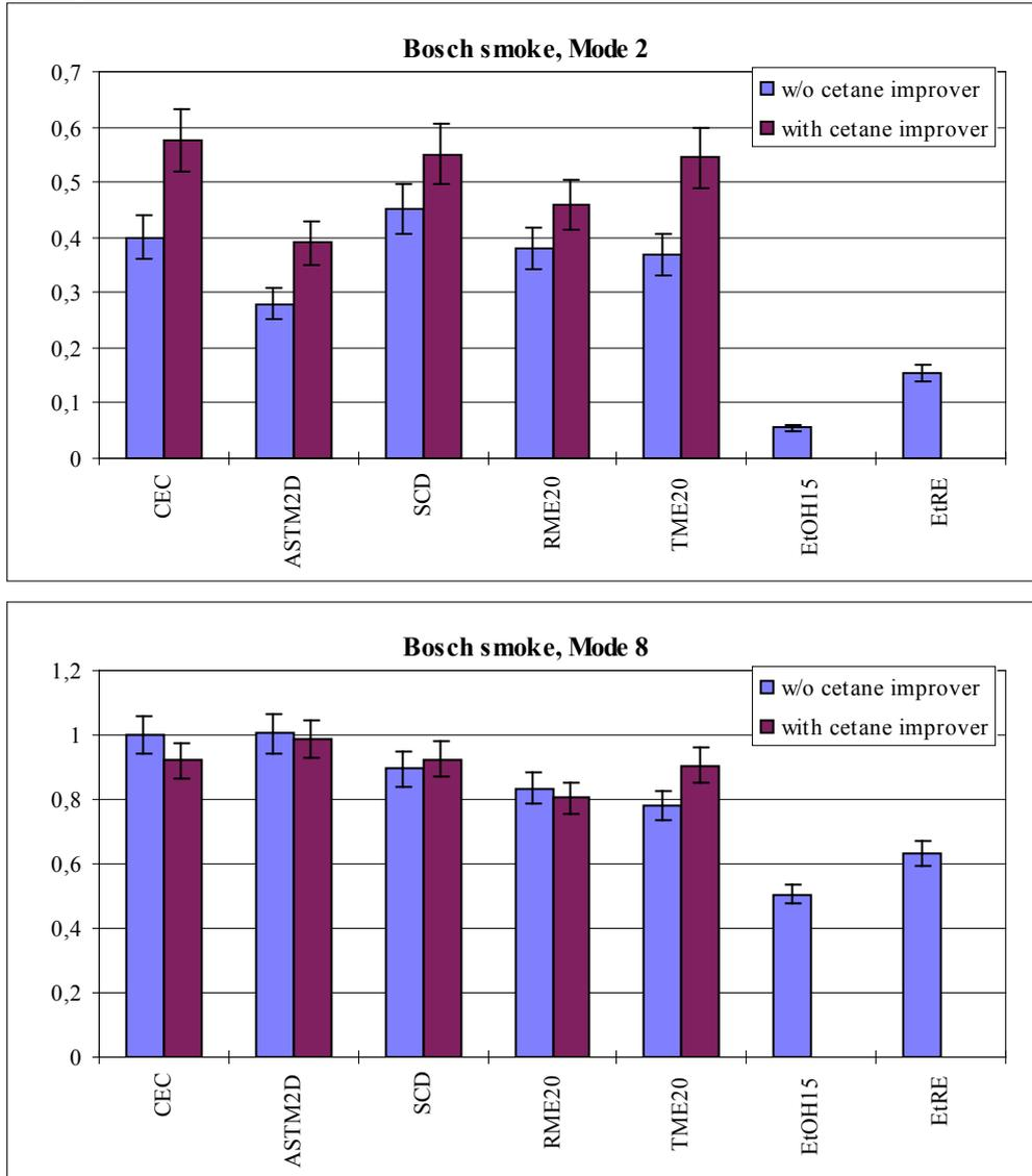
Figure 9. Bosch-smoke values with the heavy-duty VOLVO THD 103 KB engine at low load mode 2 and high load mode 8 of ECE R49 test procedure. Error bars represent standard deviations based on the highest deviations observed.
