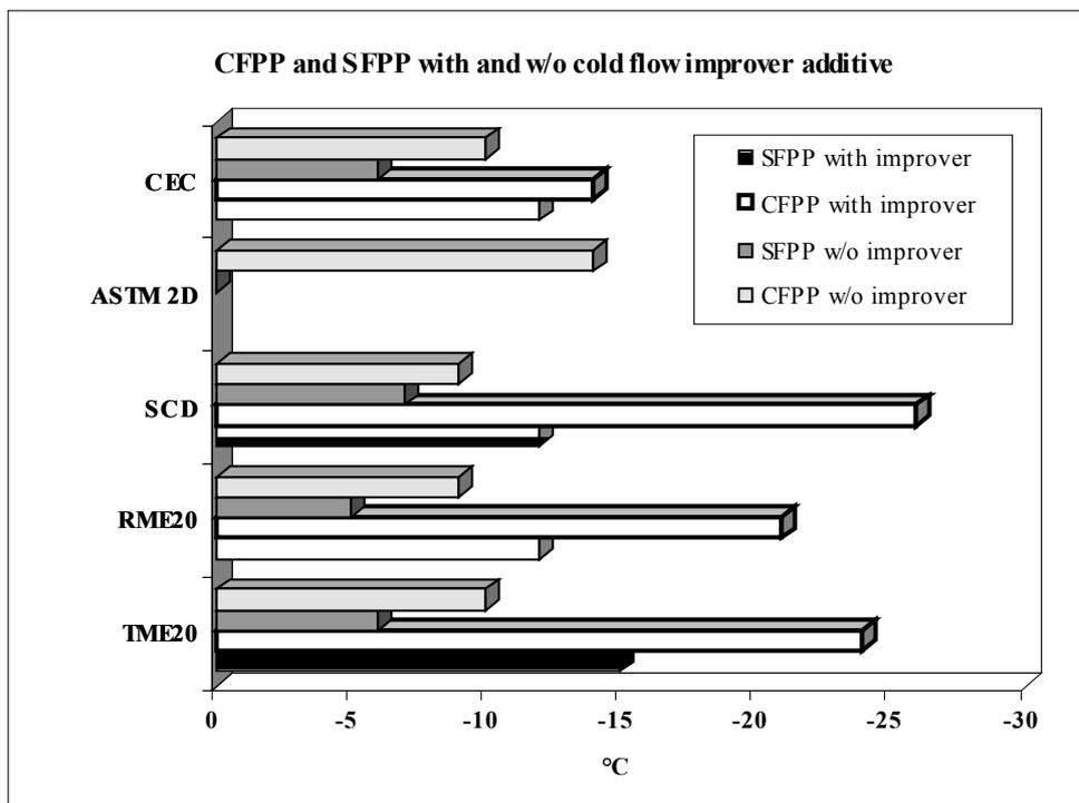
Figure 32. Cold properties of the test fuels with and without cold flow improvers.
