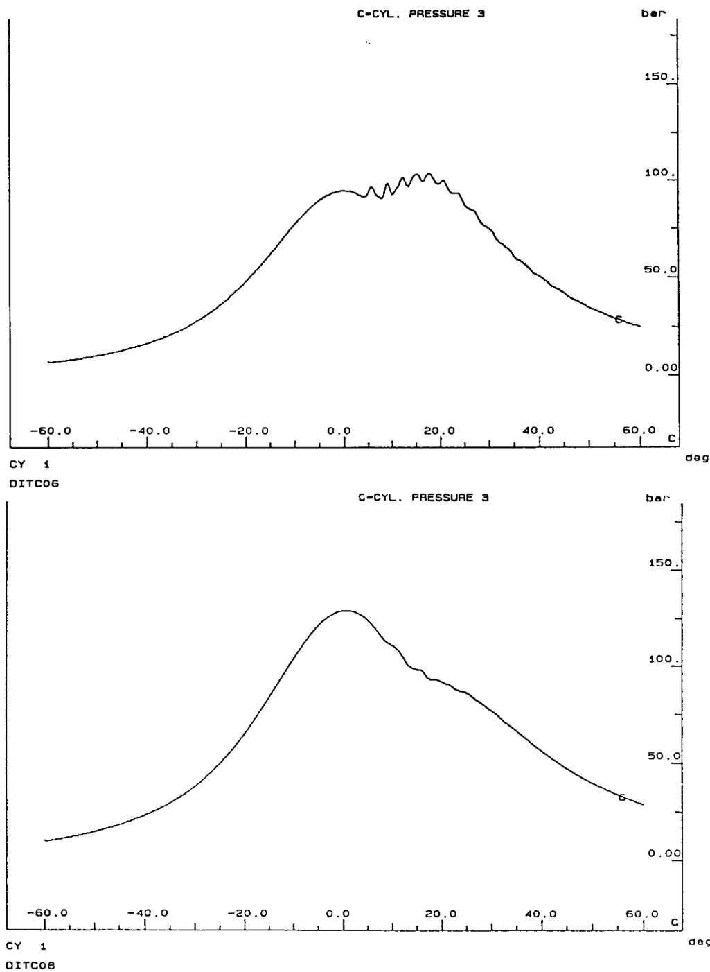
Figure 10. Cylinder pressure curves for the VOLVO THD 103 KB engine at ECE R49 modes 6 (1 300 rpm, 100% load) and 8 (2 000 rpm, 100% load).
