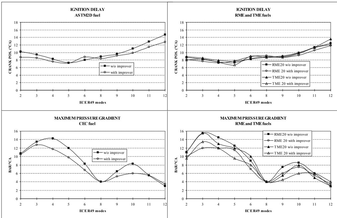
Figure 13. Ignition delay and maximum pressure gradient at different loads of ECE R49 test with the VOLVO THD 103 KB engine. Ignition delay is shorter, when the cetane improver additive is used.
