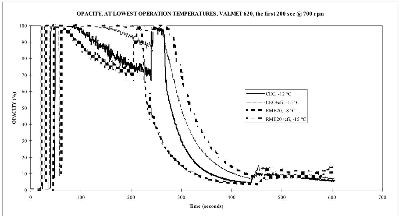
Figure 34. Opacity in the cold start test, Valmet 620.
