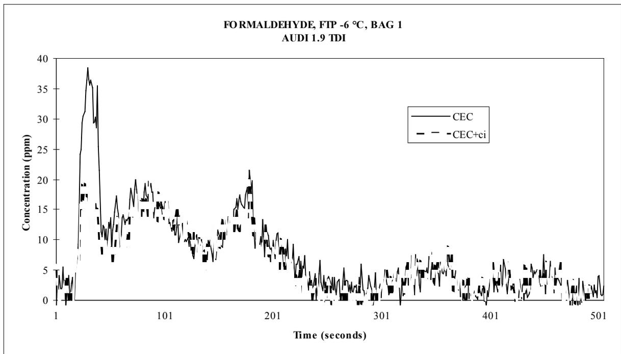
Figure 43. Formaldehyde concentrations in the first phase of the FTP test with the CEC fuel with and without the cetane improver at -6 °C. AUDI 1.9 TDI vehicle.
