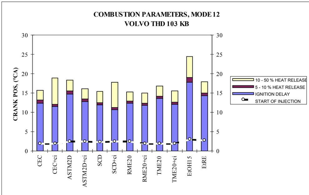
Figure 12. Combustion parameters at low load mode 2 of ECE R49 test with VOLVO THD 103 KB engine. The ignition delay is longest for the low cetane fuels.
