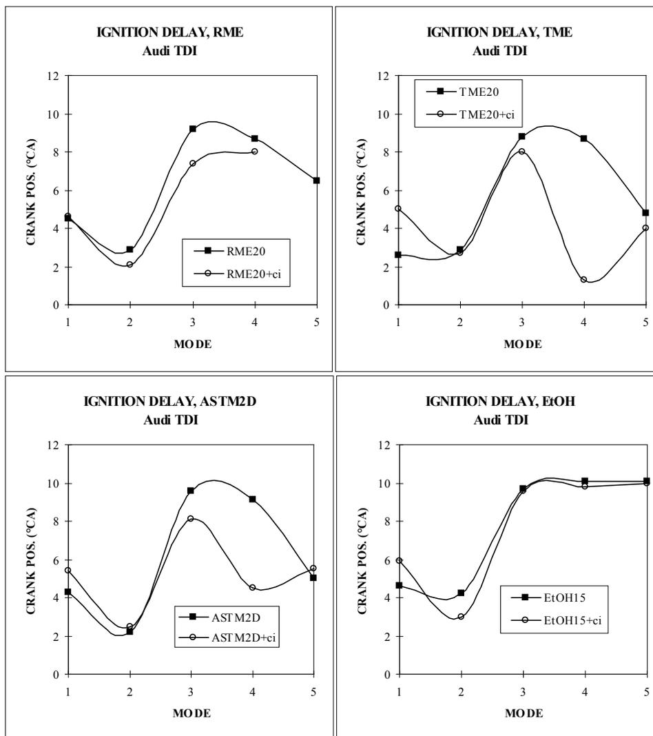
Figure 25. Some examples of the ignition delay with and without the cetane improver, Audi 1.9 TDI steady-state tests. Modes 1 and 2 mean 50 and 25% loads at rated speed. Modes 3, 4 and 5 are 100, 50 and 25% loads at intermediate speed.
