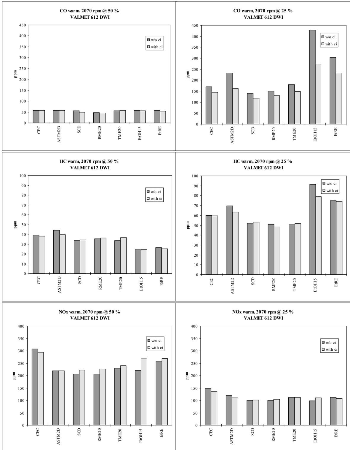
Figure 16. CO, HC and NO<sub>x</sub> concentrations at rated speed, 50 and 25% loads with the Valmet 612 DWI engine.
